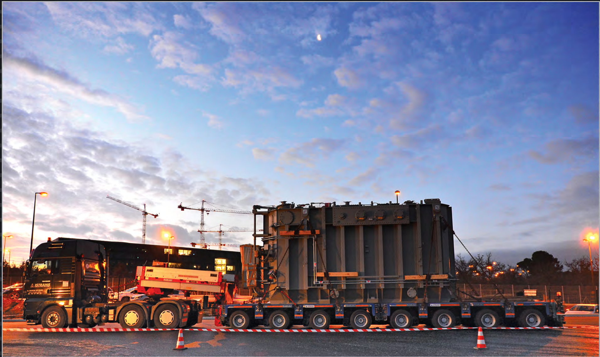
A US-procured electrical transformer is the first ITER component to be transported along the 104-km ITER Itinerary. At least 250 exceptional convoys are expected during the construction and assembly phases of ITER. January 2015
