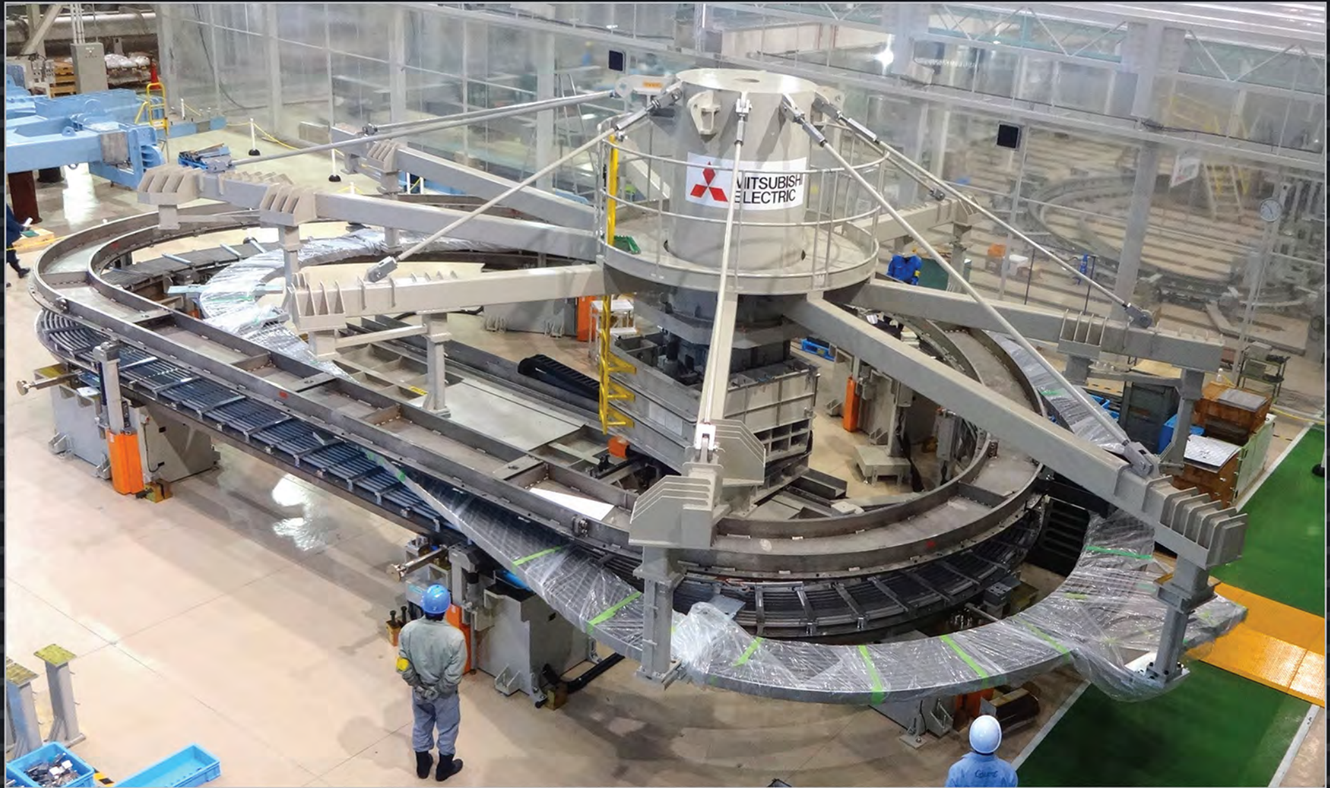
Unit lengths of conductor are wound into a D-shaped double spiral called a “double pancake” before being heat treated, electrically insulated, and finally inserted into the grooves of a radial plate. At Mitsubishi Heavy Industry’s Futami factory, transfer tooling has been successfully commissioned.
