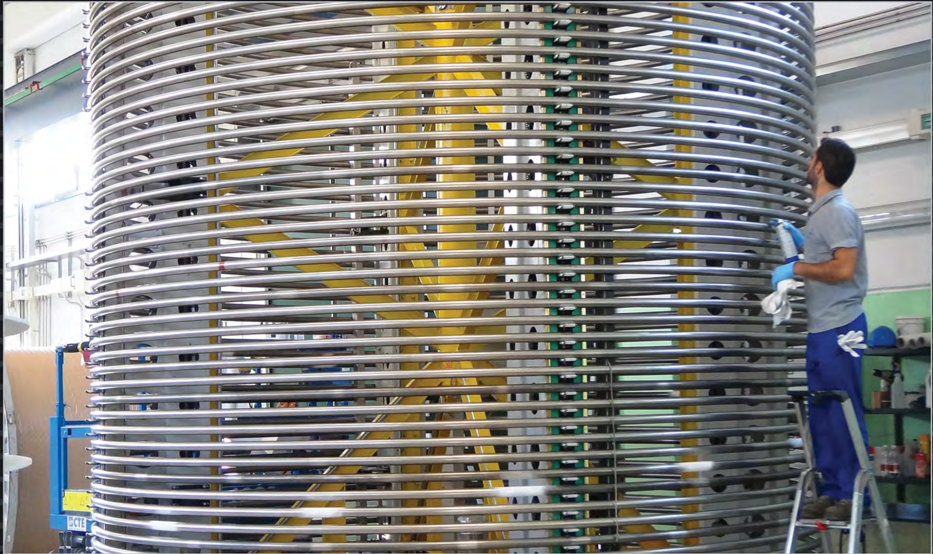
In November 2014, Korea completes all manufacturing activities for its share of toroidal field conductor (29 unit lengths).
