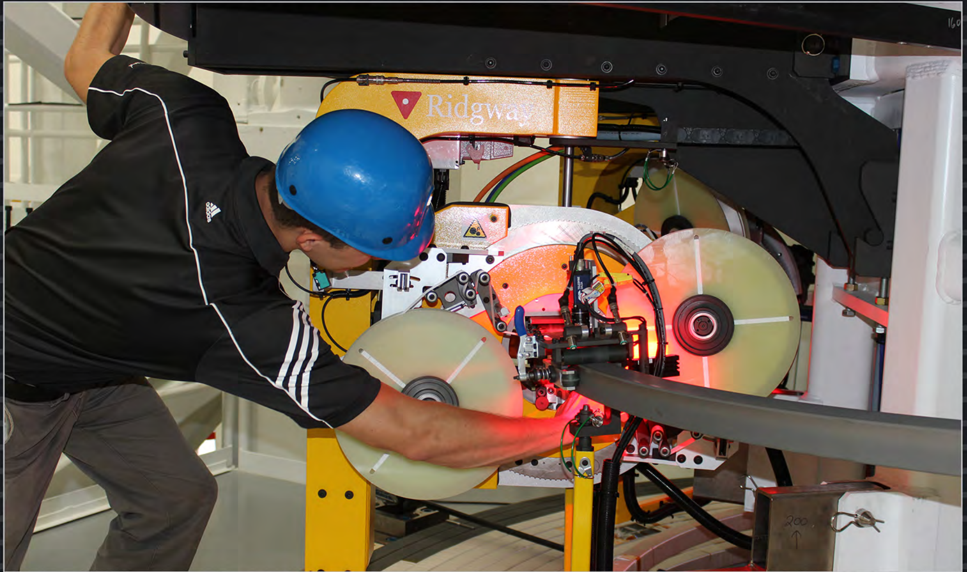
A close-up view of the central solenoid turn insulation station which will wrap fiberglass insulation around the conductor.
