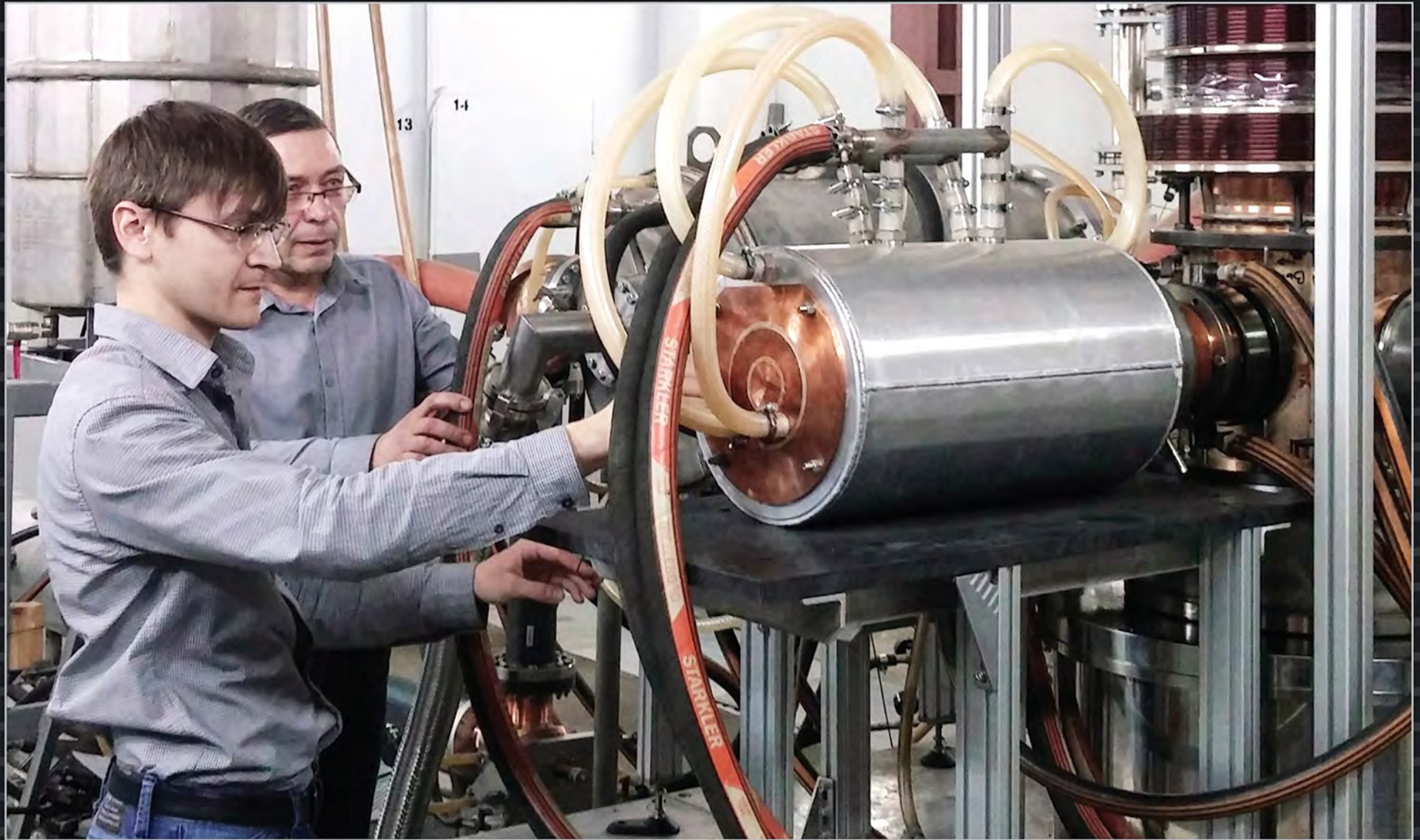
A gyrotron prototype successfully passes factory acceptance tests at Gycom Ltd in Nizhny Novgorod in May 2015. Russia is responsible for procuring 8 of the 24 energy-generating devices that will inject powerful microwave beams into the ITER vacuum vessel to heat the plasma and drive plasma current.
