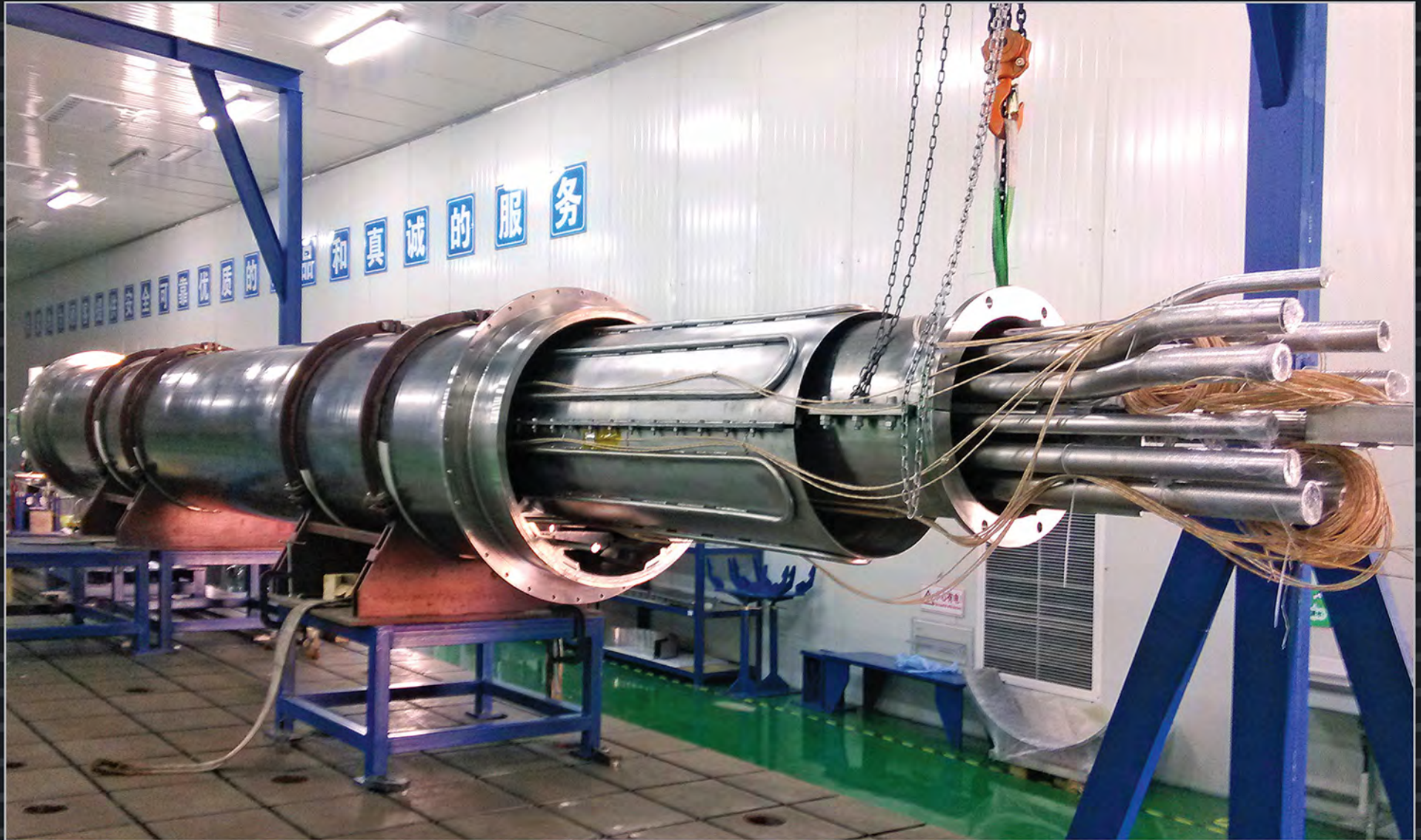
Cryostat feedthroughs cross through the cryostat and bioshield to provide a passageway to the ITER magnets for cooling pipes, power cables and instrumentation cables. This 10-metre prototype was manufactured, integrated and commissioned in November 2014 at the Institute of Plasma Physics, Chinese Academy of Sciences (ASIPP).
