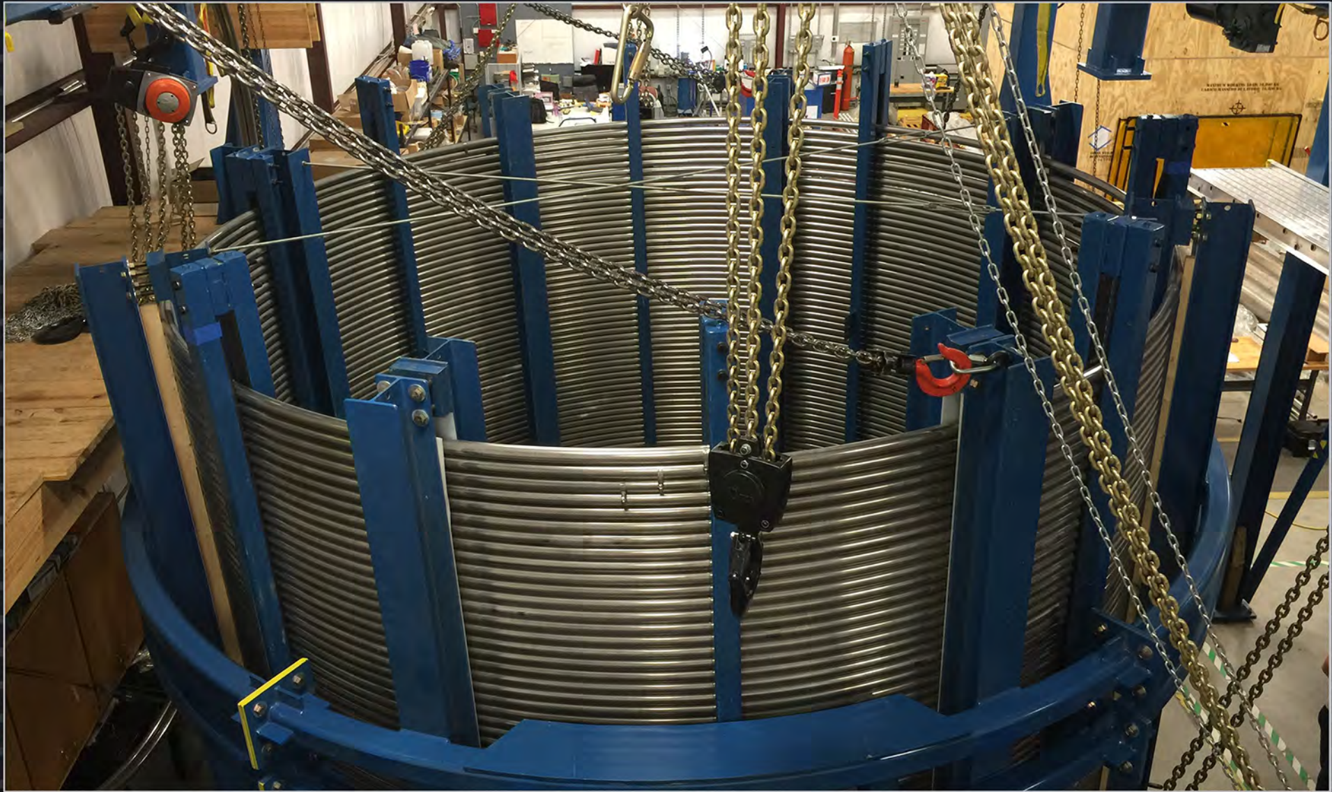
Production toroidal field conductor in the frame used to flip the conductor in preparation for shipping from High Performance Magnetics in Tallahassee, Florida.
