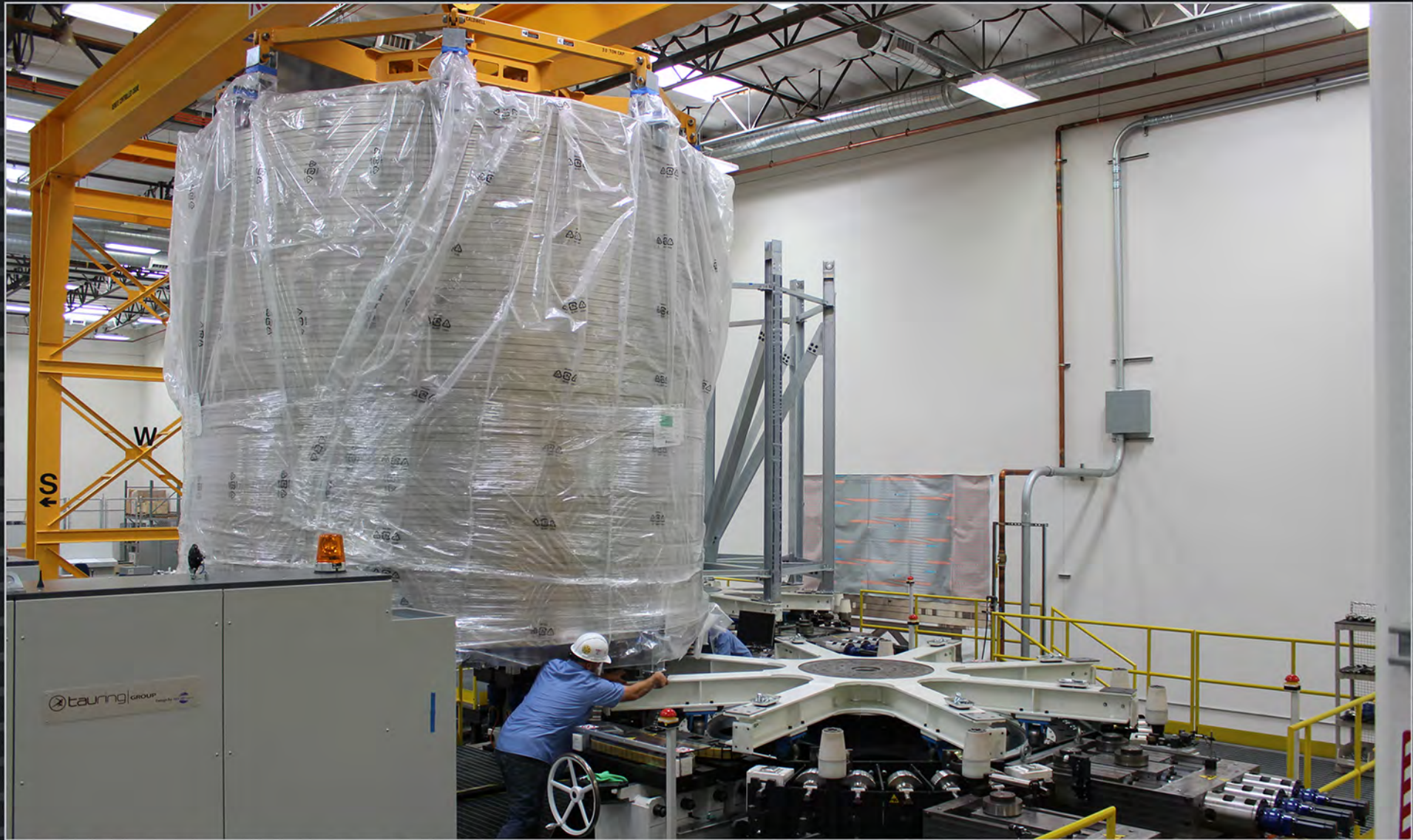
Loading conductor supplied by Japan on to the de-spooler for central solenoid module winding.
