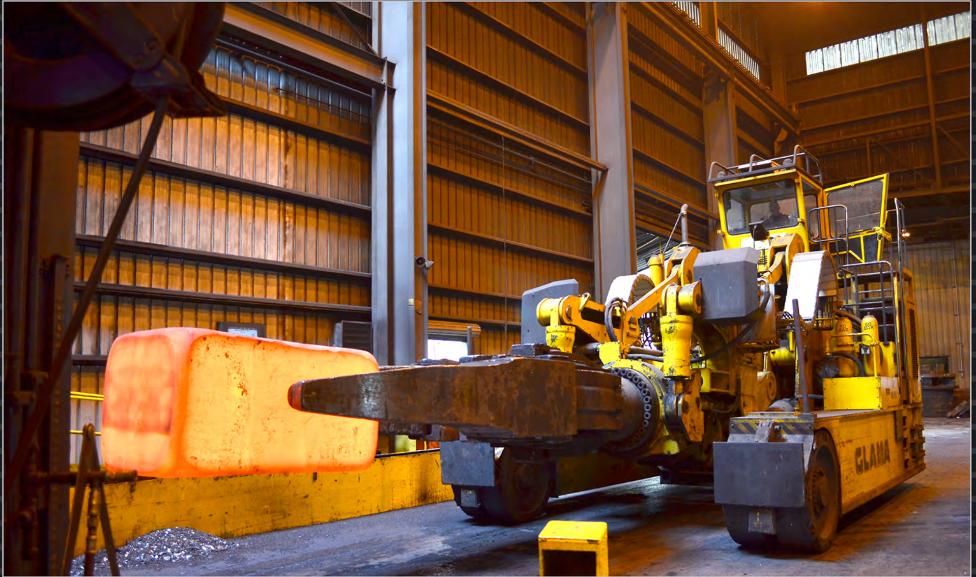
Forging of key blocks for the central solenoid at Scot Forge in Spring Grove, Illinois.
