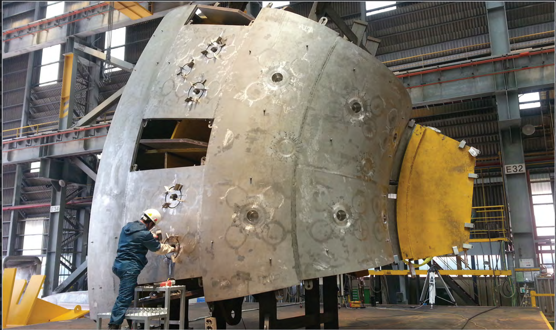
Manufacturing of the ITER vacuum vessel is underway in Korea, which is responsible for procuring two sectors out of nine. Pictured: welding operations at Hyundai Heavy Industries in Ulsan on an inner shell upper section – only a small part of one sector.
