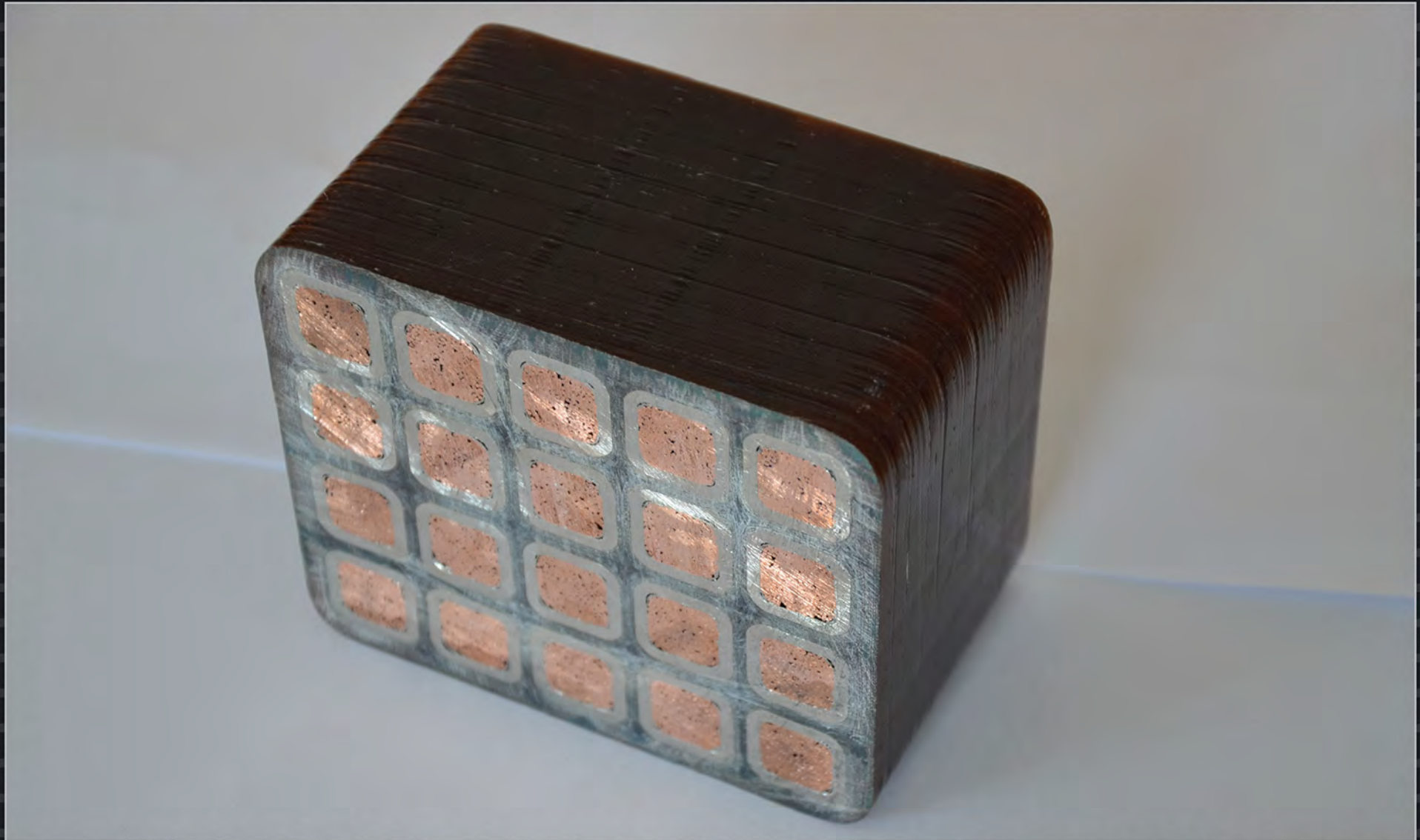
Momentum is building on the fabrication of the ITER correction coils in China. At ASIPP, a five-metre qualification length of niobium-titanium conductor has been fabricated and one prototype winding pack has been successfully manufactured and tested. (The face of the conductor sample pictured is 11 x 9 cm.)
