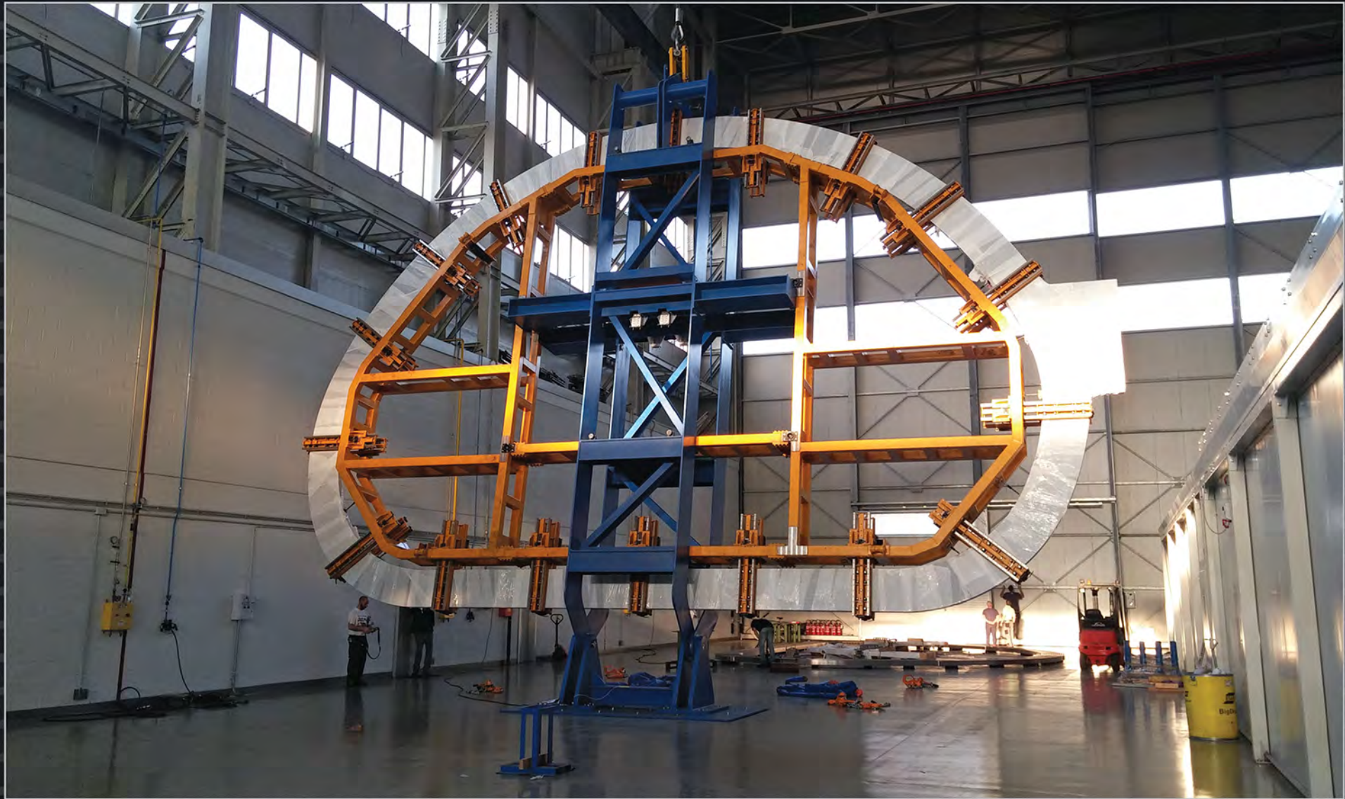
Inside of the large D-shaped toroidal field winding packs, specially grooved stainless steel radial plates, plus covers, will hold the conductor in place. In Europe, manufacturing is underway on seventy 13 x 9 m radial plates.
