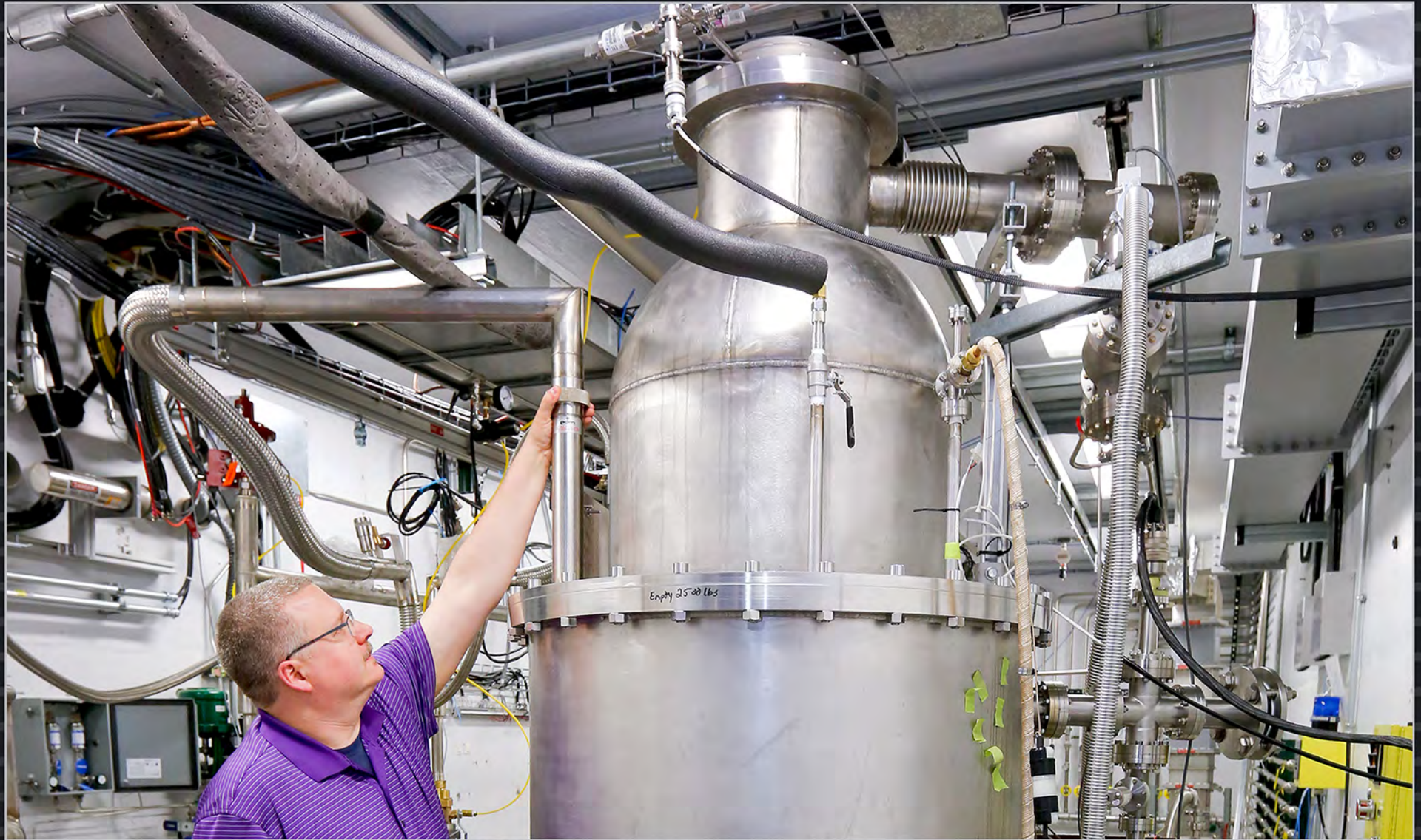
A full-scale cryoviscous compressor pump for the vacuum auxiliary system was manufactured by Major Tool in Indianapolis, Indiana and tested at the Cryogenic Testing Facility of the Spallation Neutron Source at Oak Ridge National Laboratory.
