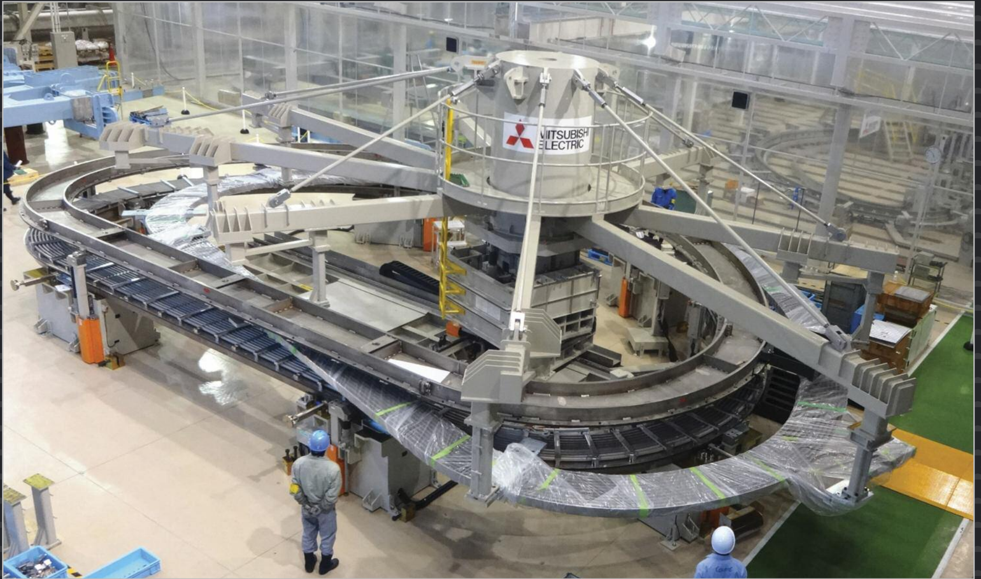
Unit lengths of conductor are wound into a D-shaped double spiral called a “double pancake” before being heat treated, electrically insulated, and finally inserted into the grooves of a radial plate. At Mitsubishi Heavy Industry’s Futami factory, transfer tooling has been successfully commissioned.
