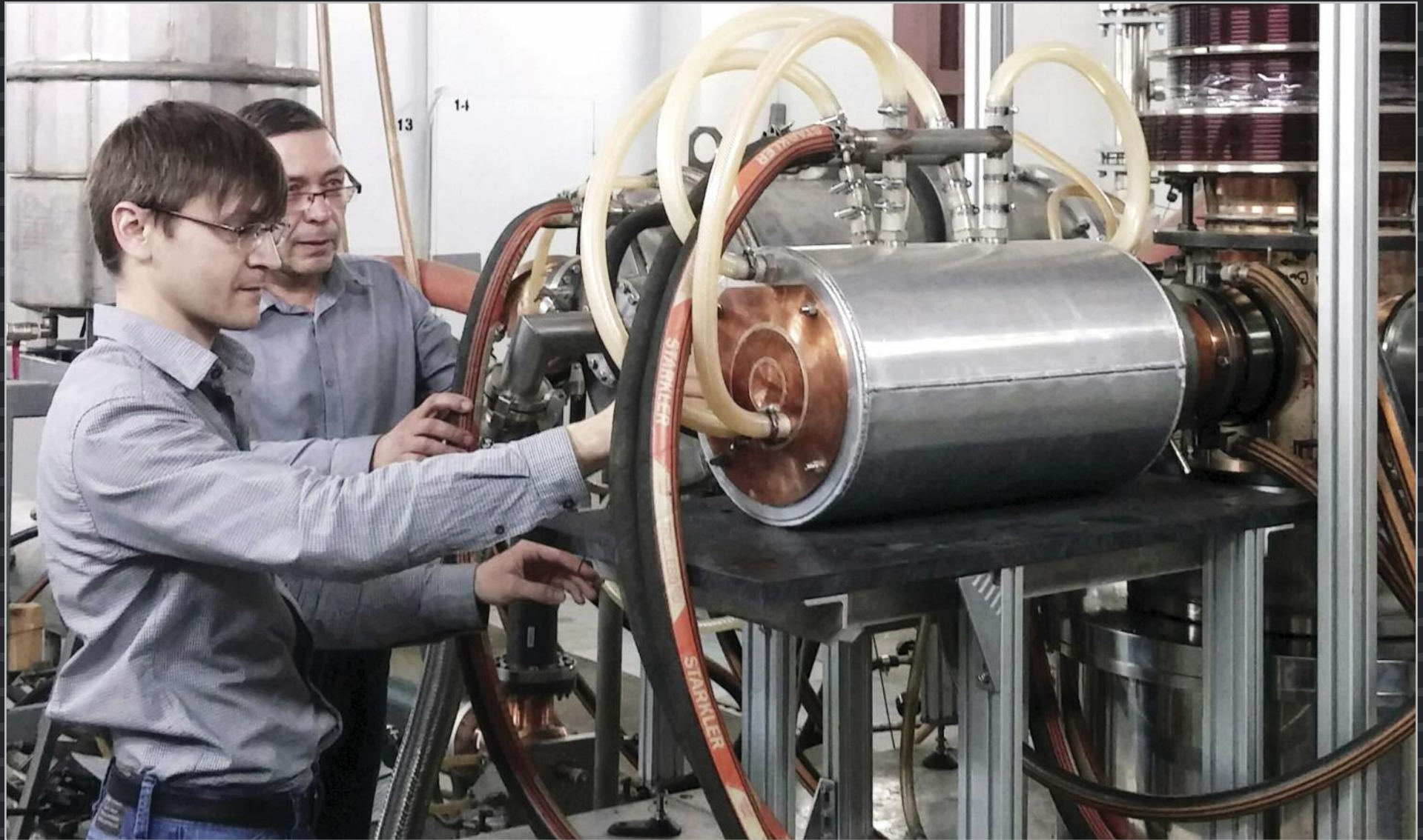
A gyrotron prototype successfully passes factory acceptance tests at Gycom Ltd in Nizhny Novgorod in May 2015. Russia is responsible for procuring 8 of the 24 energy-generating devices that will inject powerful microwave beams into the ITER vacuum vessel to heat the plasma and drive plasma current.
