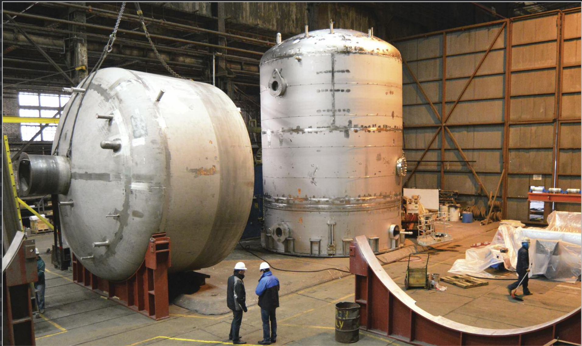
Five drain tanks for ITER's tokamak cooling water system have been successfully fabricated at the Joseph Oat Corporation in Camden, New Jersey and shipped to the ITER site. The tanks arrived in two convoys (May and September 2015).
