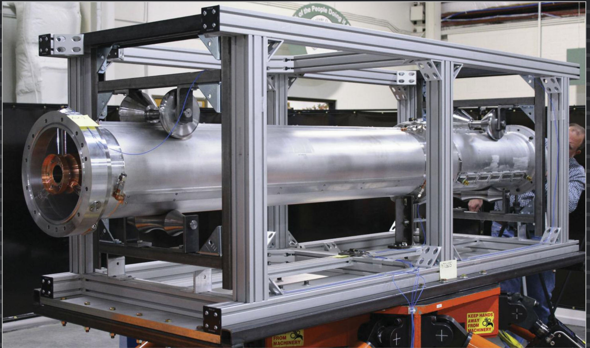
The ion cyclotron system heats the ions in the plasma with a high-intensity beam of electromagnetic radiation. In the US, an ion cyclotron transmission line prototype undergoes seismic testing.
