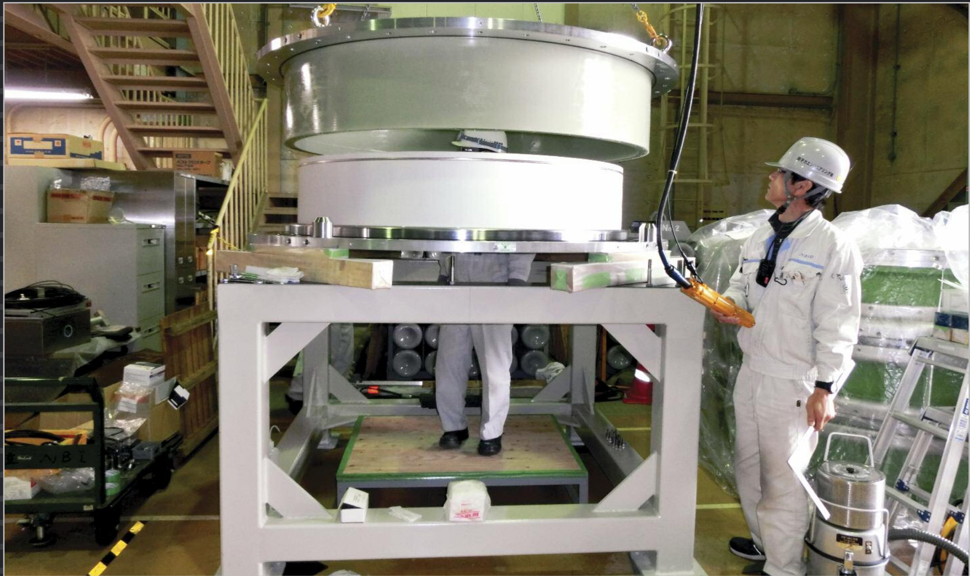
Ceramic bushing rings serve as insulators on ITER's neutral beam heating system, connecting the high pressure transmission lines for the 1 MV power supply with the vacuum chamber inside the system. This one, assembled at the Japan Atomic Energy Agency with an outer tube in fibre-reinforced plastic, has a diameter of 1.56 metres, making it the largest in the world.
