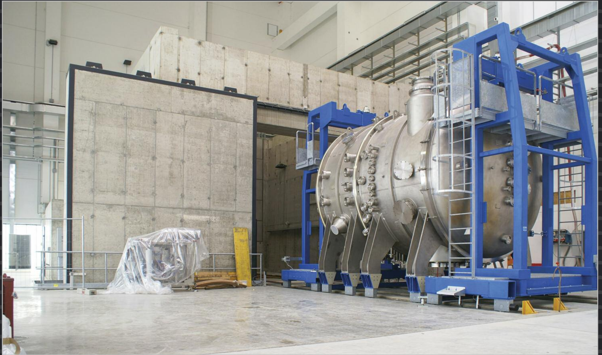
At the PRIMA facility in Padua, Italy, ITER neutral beam technology will be tested in advance of operation on SPIDER (an ITER-scale radio-frequency negative ion source) and MITICA (a full-scale ITER neutral beam injector at full acceleration voltage and power). Europe, Japan and India are all contributing components. In 2015, Europe delivered the SPIDER vacuum vessel pictured above.
