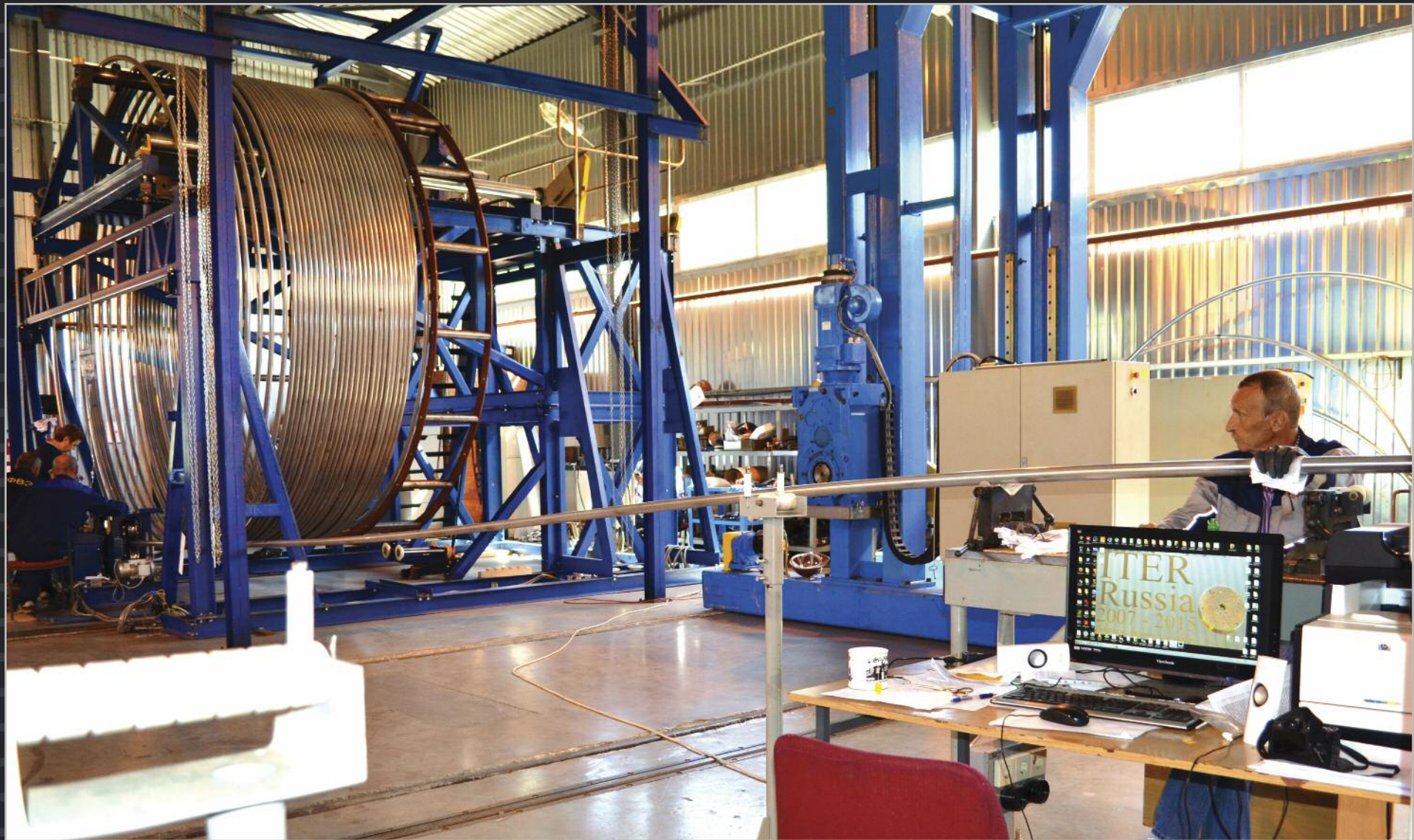
At the Institute of High Energy Physics in Protvino, Russia, the last production lengths of toroidal field conductor are jacketed and compacted in June 2015. This marks the end of a five-year campaign to manufacture 28 production lengths, or more than 120 tonnes of material, for ITER's toroidal field coils.
