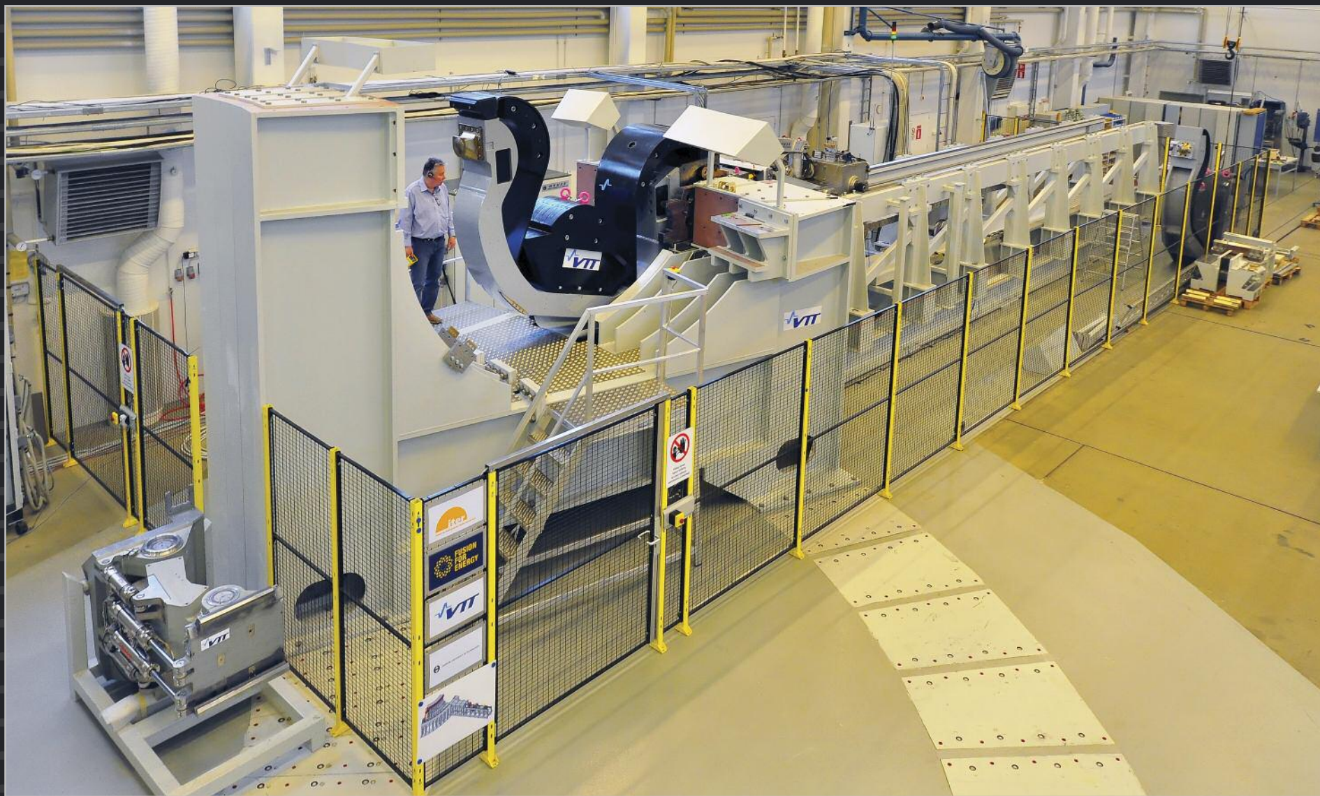
Europe is responsible for procuring the remote handling systems for the ITER divertor, the neutral beam, the cask transfer system, and the in-vessel viewing and metrology system. Pictured: the final demonstration of divertor cassette remote handling is successfully performed in 2015 at the DTP2 Divertor Test Platform facility in Tampere, Finland.
