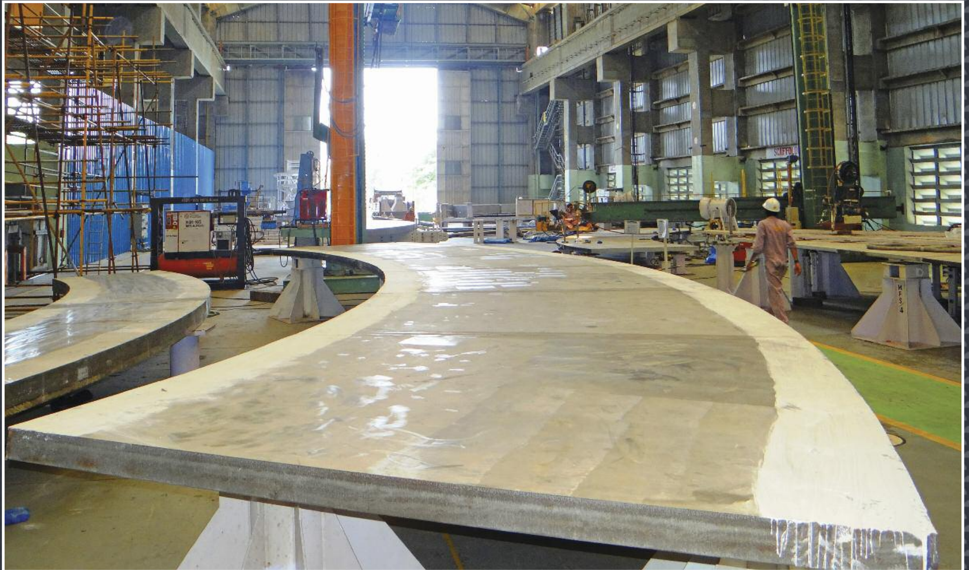
In Hazira, on the northwestern coast of India, fabrication of real-scale prototypes for the cryostat has begun. Pictured here is a portion of the horizontal plate (60° sector) for the cryostat base section, made of 105-mm-thick stainless steel.
