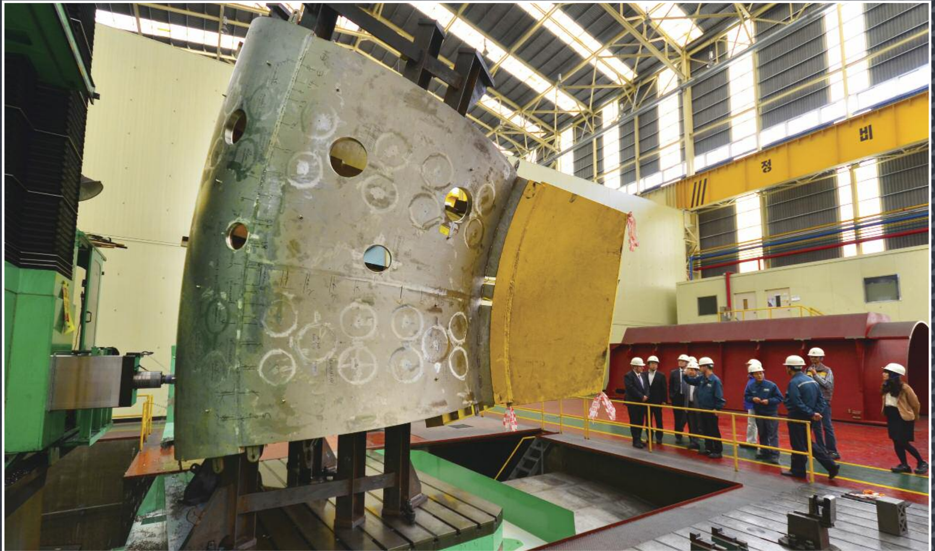
Manufacturing of the ITER vacuum vessel sectors is underway in Korea, which is responsible for procuring two sectors out of nine. Pictured is the upper segment of Sector #6, made of special ITER-grade steel, at Hyundai Heavy Industries in Ulsan, South Korea.
