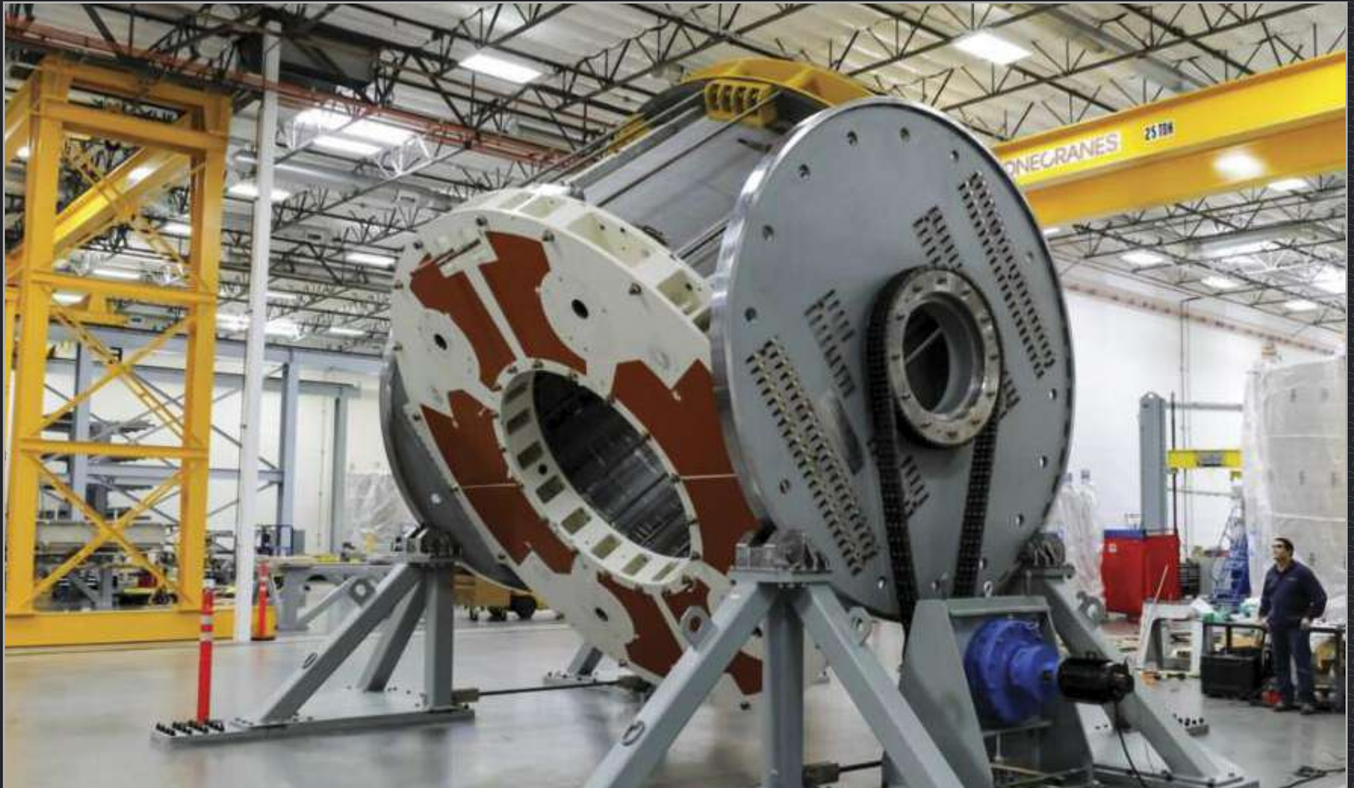
At different stages of fabrication, the top or bottom of a central solenoid module must be accessible. This turnover tool makes easy work offloading the 110-tonne components.
