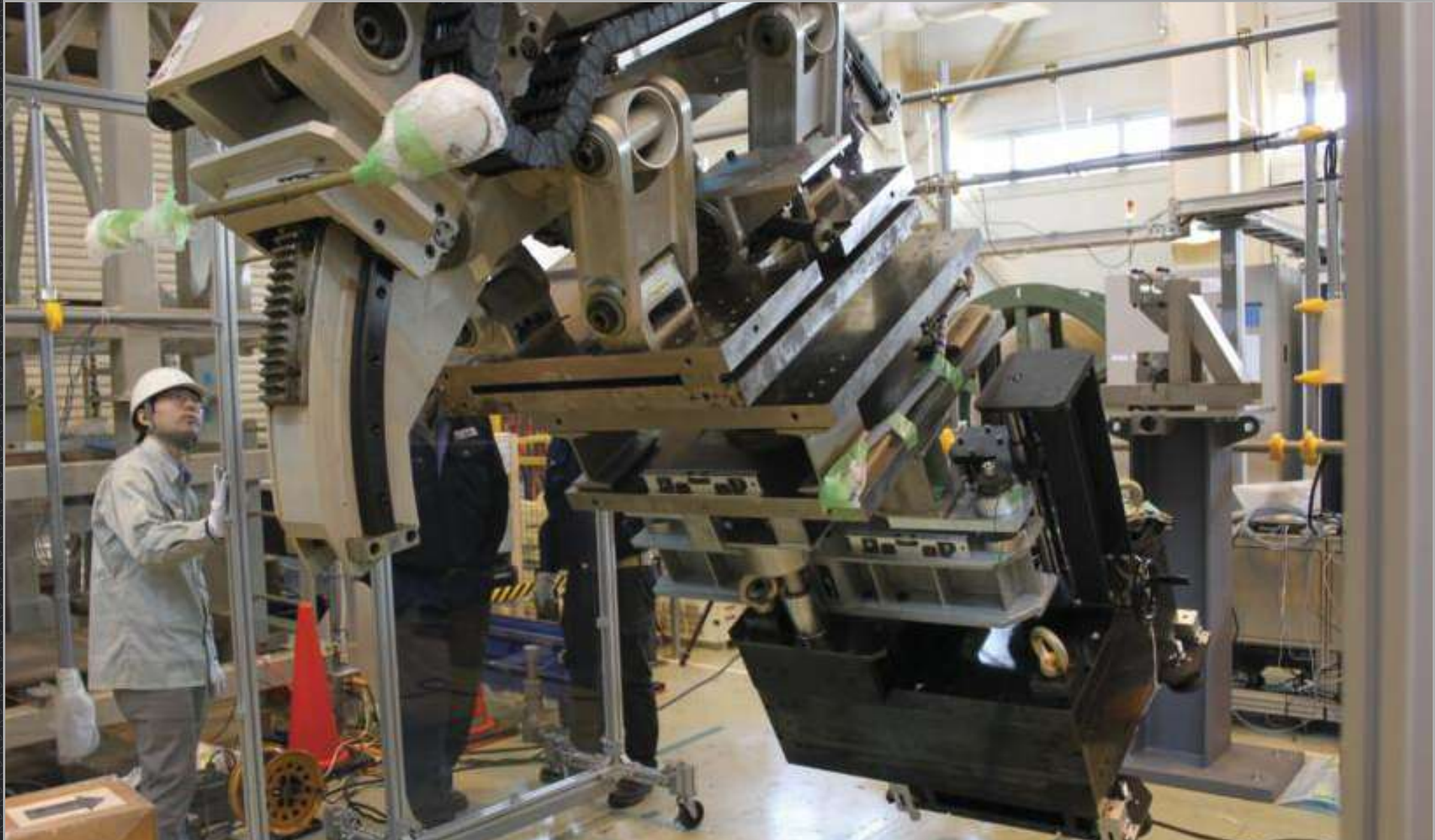
Although not as powerful as the Infinity Gauntlet of comic book fame, the bolting tool (pictured) that will be used to install ITER's in-vessel blanket modules robotically is impressive. It will provide 10 kilonewton metres (kNm) of torque to tighten the massive bolts of the blanket first wall panels remotely.
