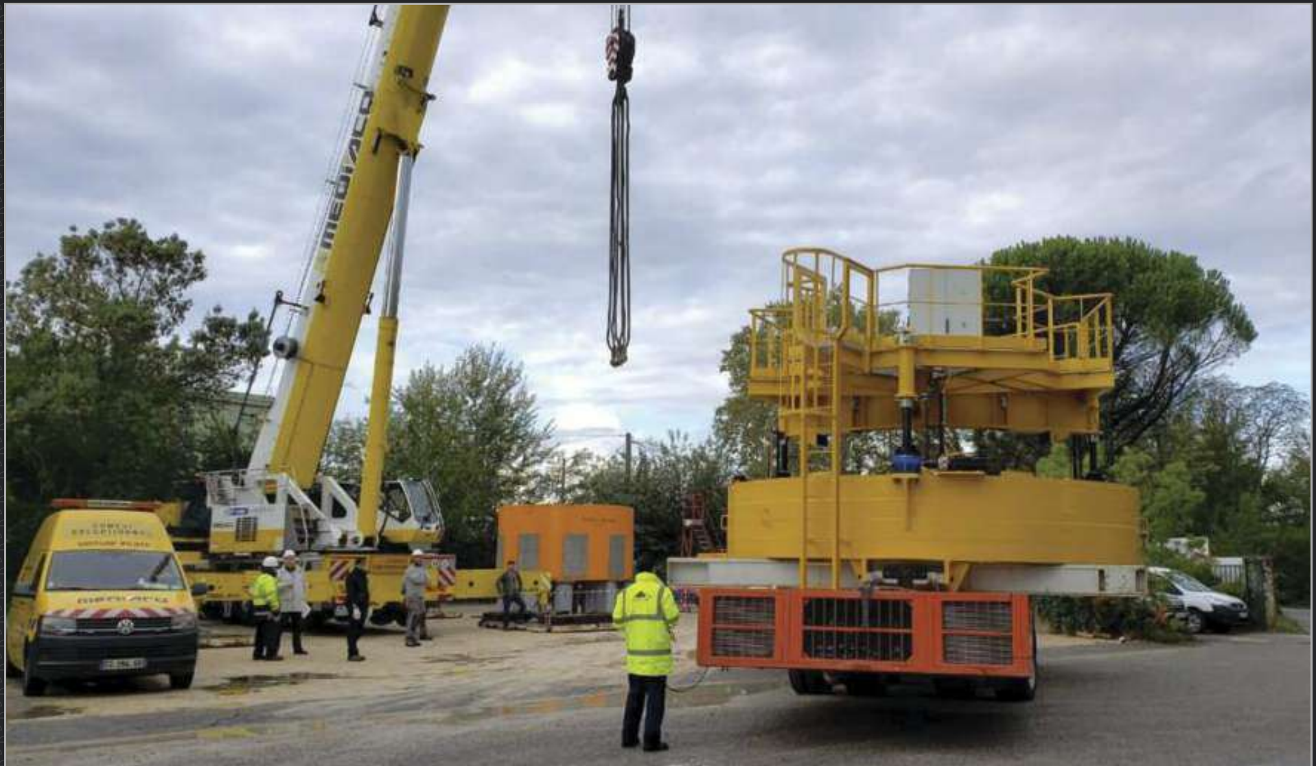
Factory acceptance testing of the central solenoid module lifting fixture is underway in Bouc Bel Air, France. The 18-metre-tall electromagnet will be assembled in the ITER Assembly Hall using tooling supplied by US ITER.
