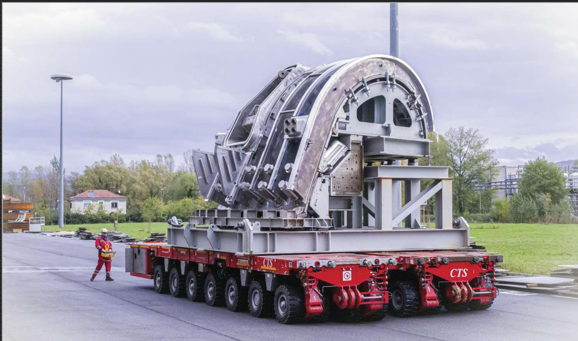
Fusion for Energy, the European Domestic Agency, is delivering five of ITER's nine vacuum vessel sectors. The first to come off the production line will be Sector #5. (Pictured, the lower poloidal segment of Sector #5 as it enters a facility for radiographic tests.)
