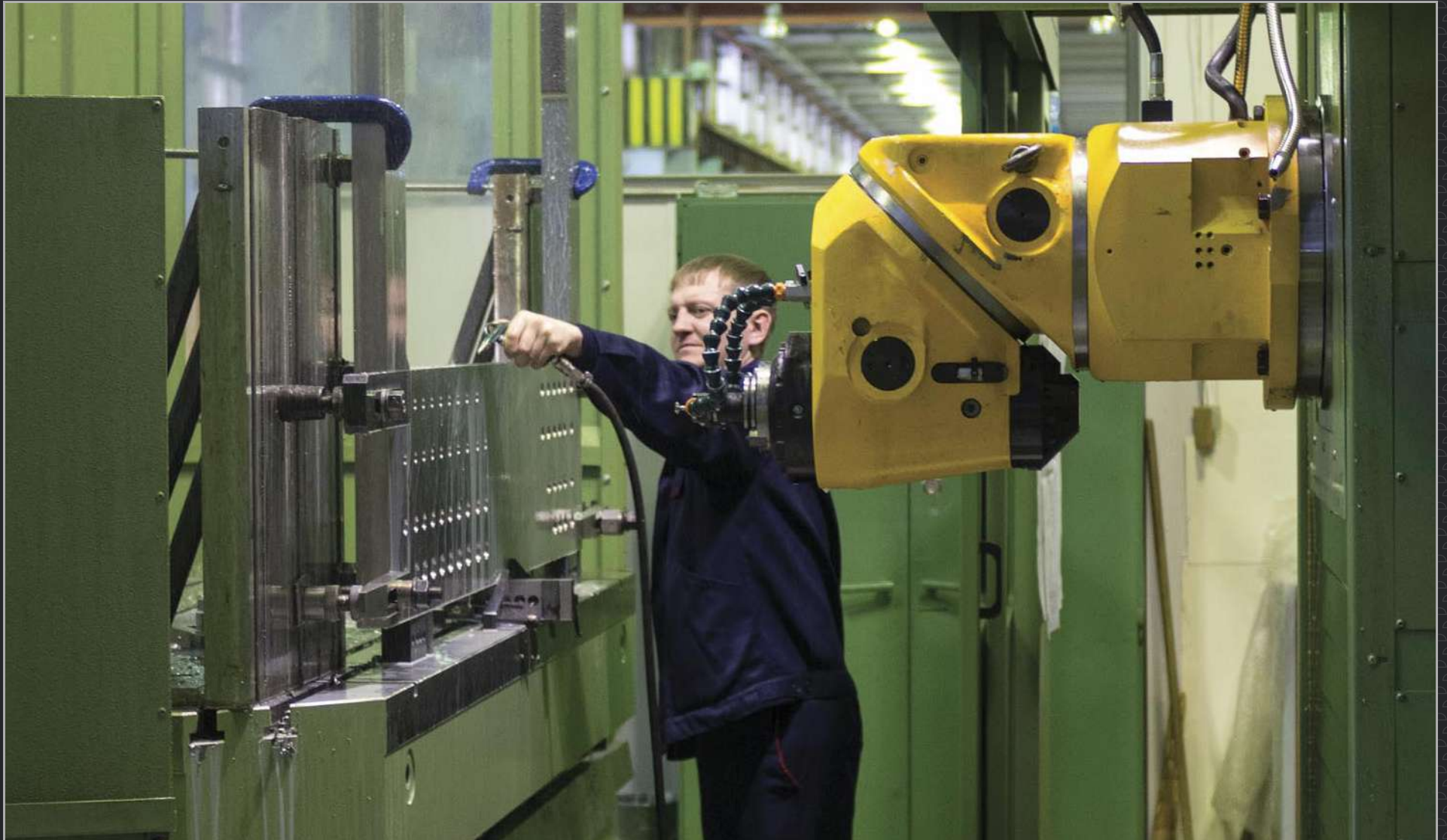
Many of ITER's diagnostics will be mounted in the port openings of the vacuum vessel, supported within "port plugs," and integrated into drawer-like structures called diagnostic shielding modules. Russian contractors are currently developing production technologies through mock-ups.
