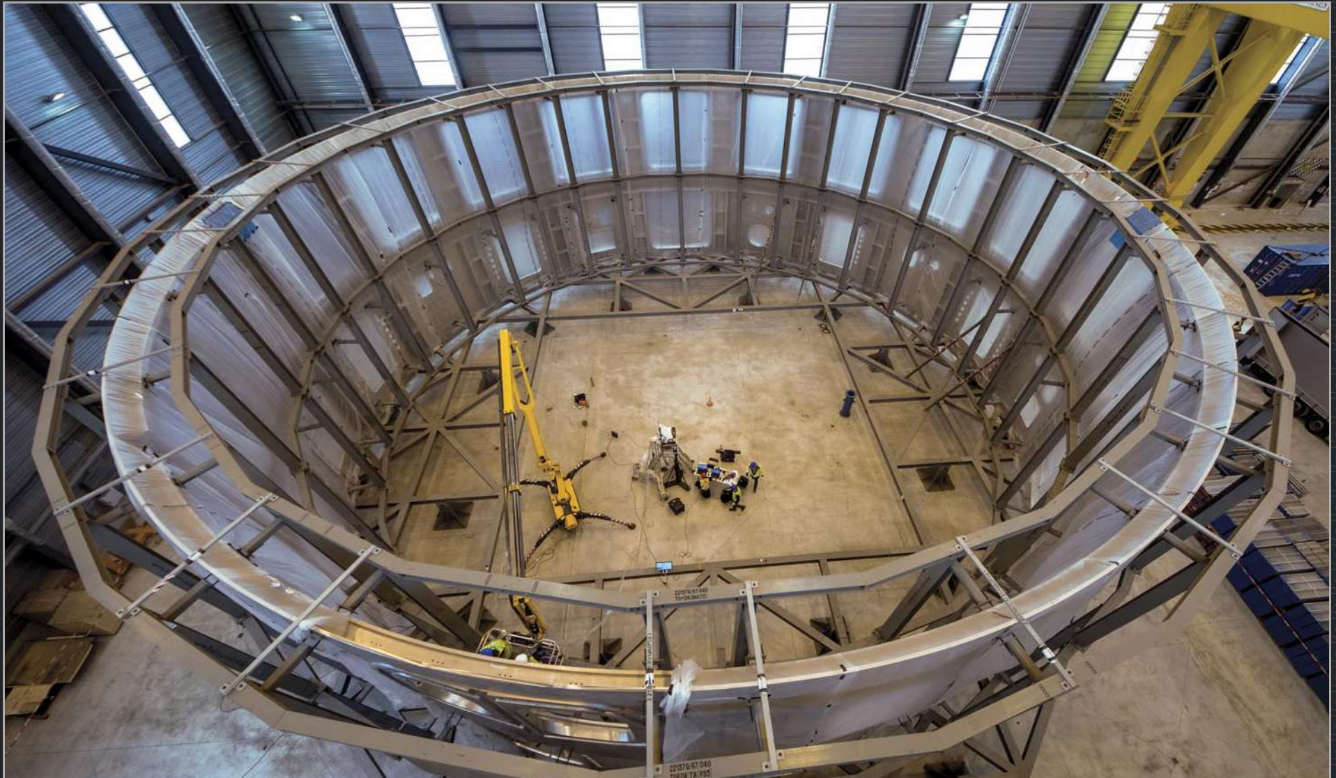
The Indian Domestic Agency delivers half of the ITER cryostat in 2019 – the 490-tonne lower cylinder (pictured) and the 1,250-tonne base. The lower cylinder has since been removed from the workshop on its platform and stored in order to make room for the assembly of the upper cylinder.
