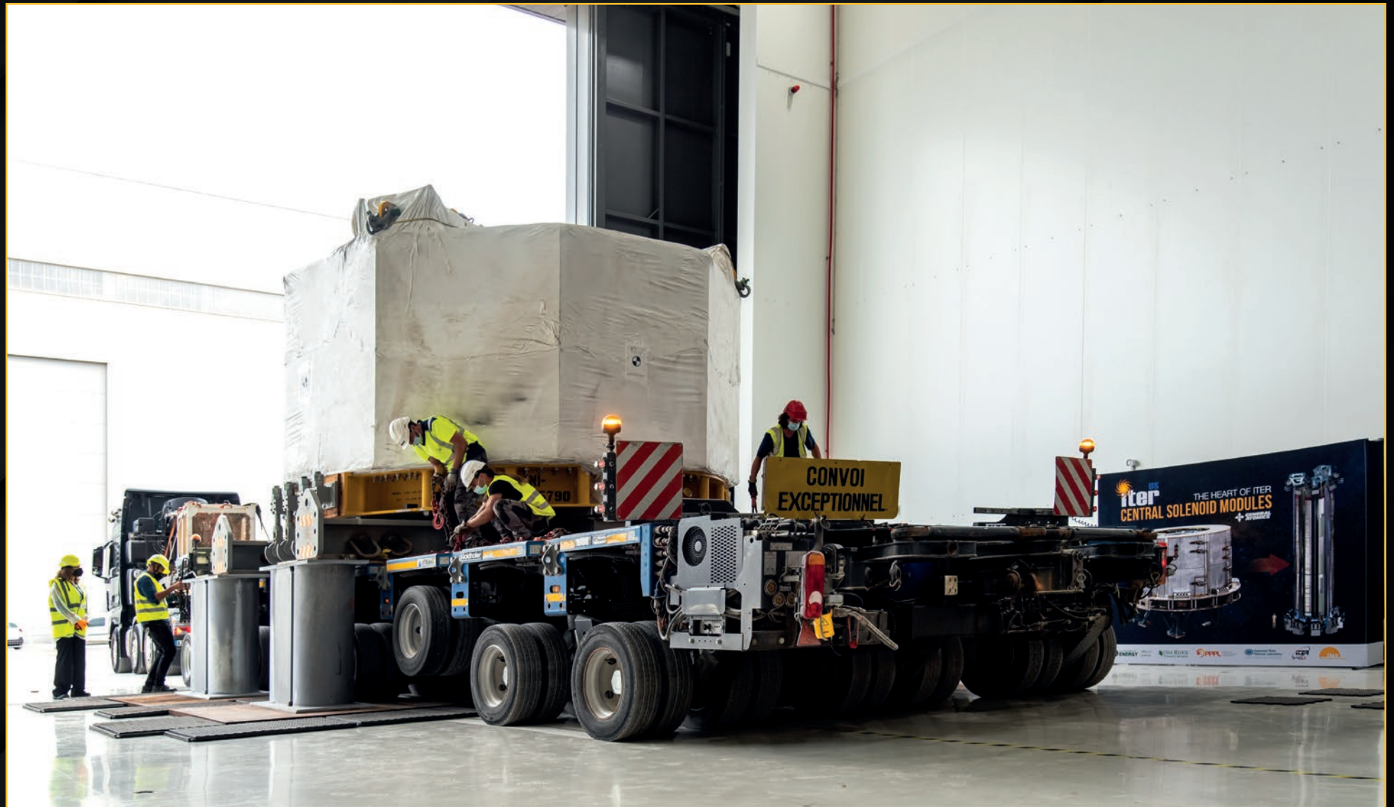
Another Highly Exceptional Load (HEL) delivered to ITER in 2021 is this central solenoid module from the United States. The ITER Organization has received 138 HELs since 2015, including 34 in 2021. September 2021
