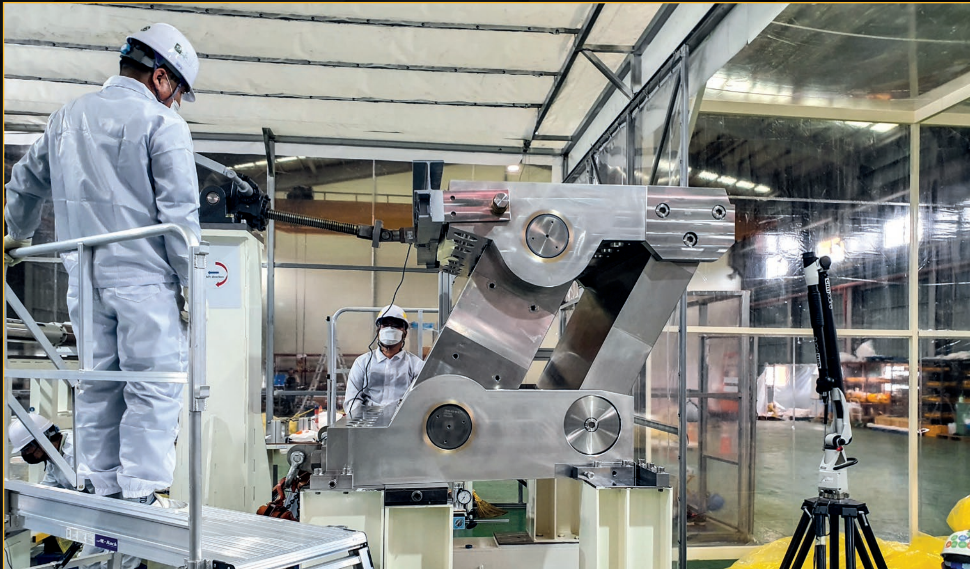
The factory acceptance test on the first ITER vacuum vessel gravity support has been successfully completed at Haneul Engineering in Gunsan, Korea. Under the plasma chamber, nine gravity supports will allow for the vacuum vessel's thermal expansion and sustain loads in the radial, toroidal and vertical directions.
