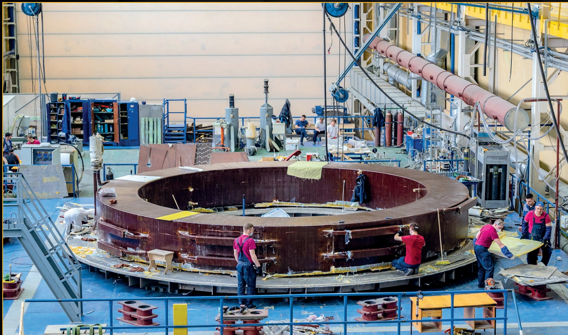
In early 2021, Russian specialists complete the vacuum pressure impregnation of poloidal field coil #1 (PF1), conferring electrical insulation with extremely high dielectric and mechanical strength to the component. In March 2022, the magnet successfully passes all factory tests.
