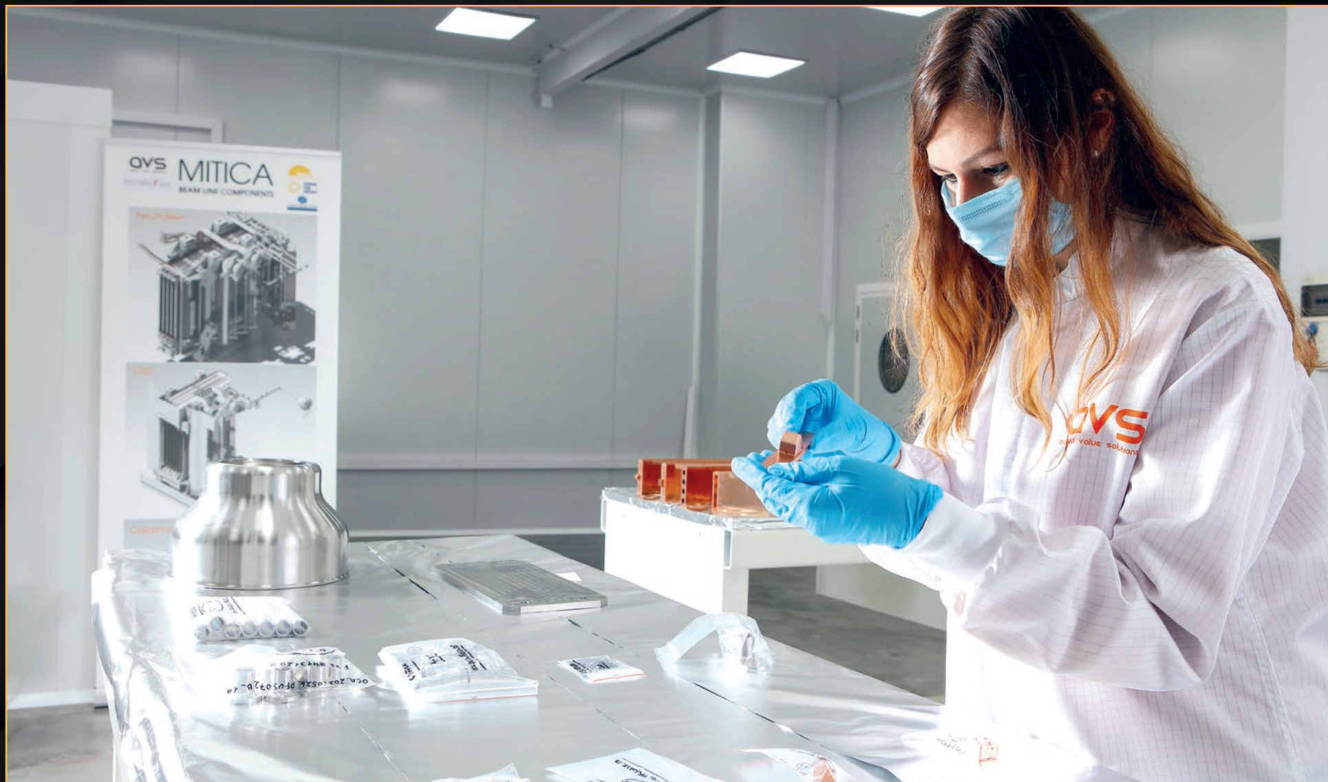
Planned for ITER's Neutral Beam Test Facility in Italy, the MITICA testbed (for Megavolt ITER Injector and Concept Advancement) is a full-size prototype of the project's 1 MV heating neutral beam injectors, capable of full acceleration voltage and power. Europe is procuring the beam source, including the beam stop elements under inspection in this image.
