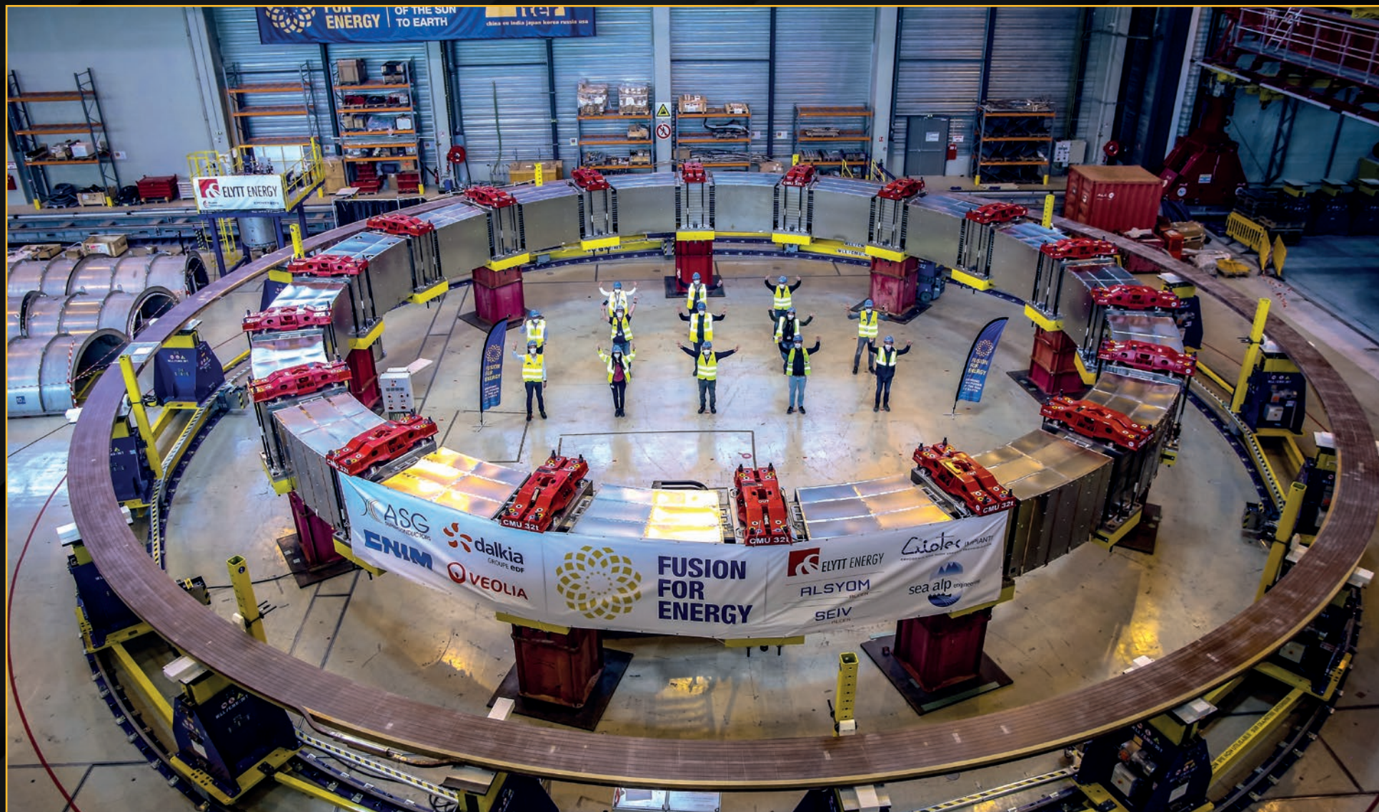
Arms are lifted in triumph as the first poloidal field coil produced by European contractors in the on-site winding facility, PF5, passes all testing. A second coil (PF2) is completed in December. April 2021
