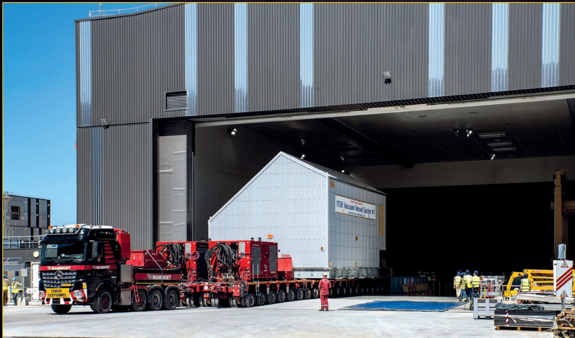
A second vacuum vessel sector (#1(7)) arrives from Korea in August. The nine 40-degree sectors required to form the ITER toroidal chamber are largely similar, differing only in the details relevant to their position in the circular arrangement and interfacing components. August 2021
