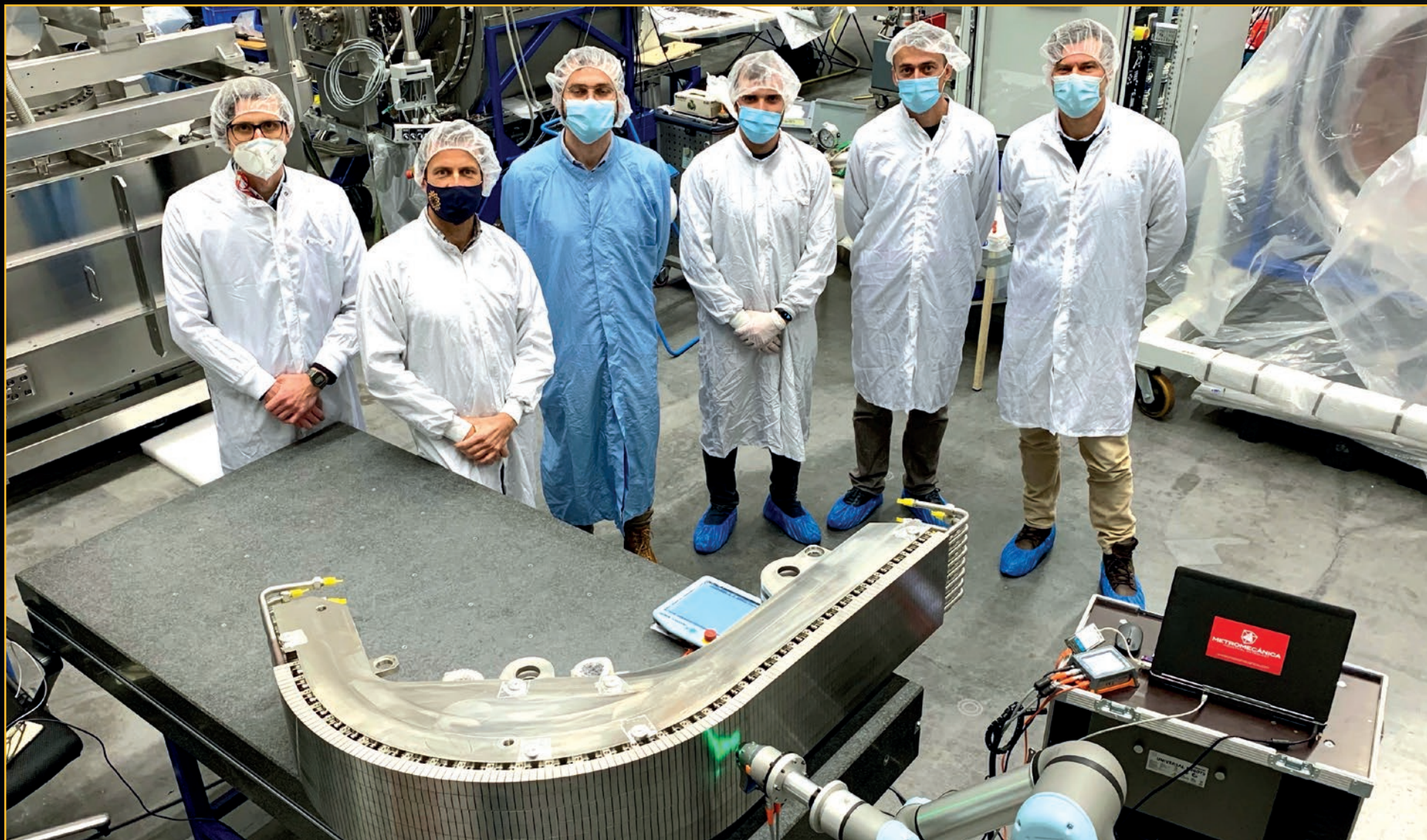
Representatives of Fusion for Energy (F4E), Research Instruments, and Metromecanica observe dimensional tests on a full-scale divertor inner vertical target prototype. The target's surface is made of small monoblocks in tungsten, which can withstand some of the highest heat loads of the ITER machine.
