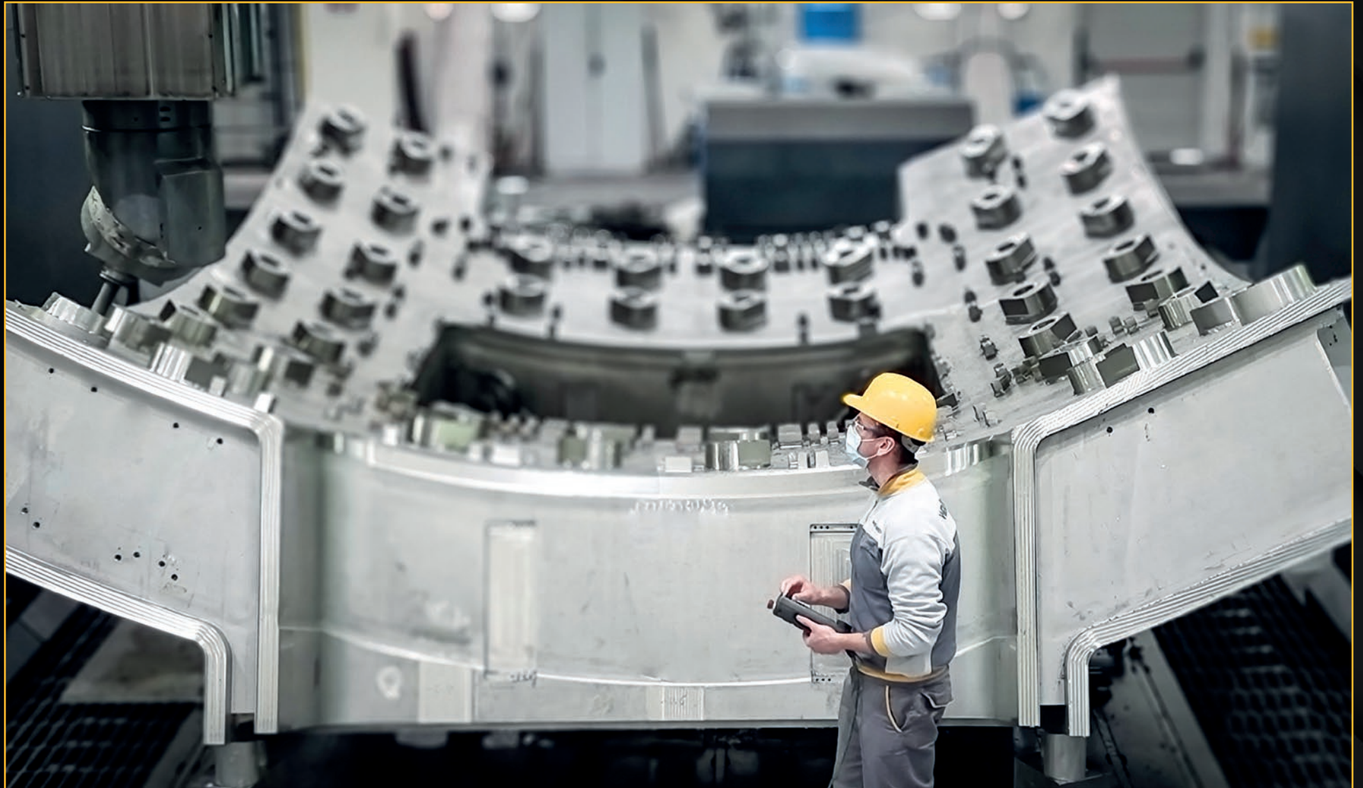
The European Domestic Agency, Fusion for Energy (F4E), is procuring five vacuum vessel sectors as part of its in-kind contributions. The first to be delivered to ITER (sector #5, pictured) is over 96% complete.
