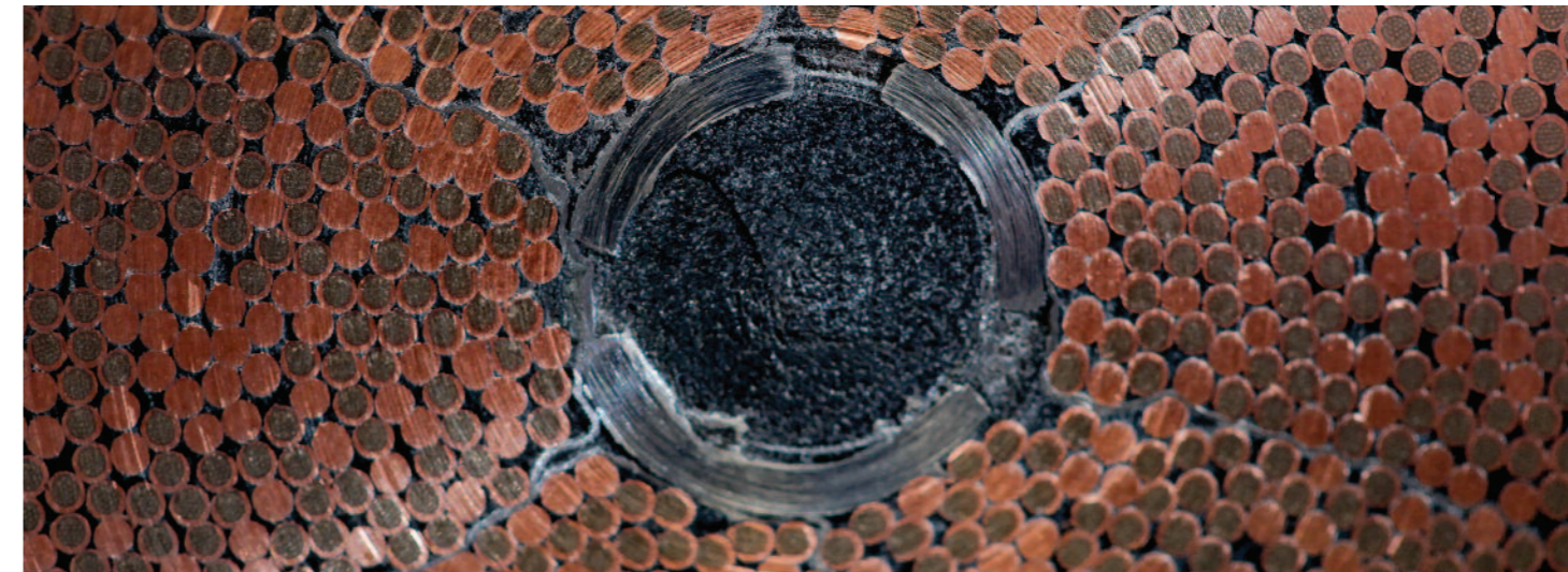
Close-up of a compacted sintered joint developed for the central solenoid magnet system. Individual superconducting strands, interspersed with copper strands, surround the central cooling channel. Photo: US ITER
