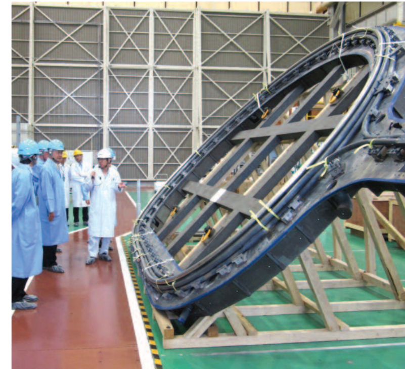
The mockup section of a toroidal field coil case. Photo: Toshiba, Keihin Product Operations, Yokohama, Japan.
