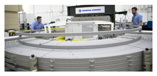
U.S. Winding of  $2^{nd}$  Central Solenoid Superconducting Magnet Production Module (Credit: General Atomics, Inc)
