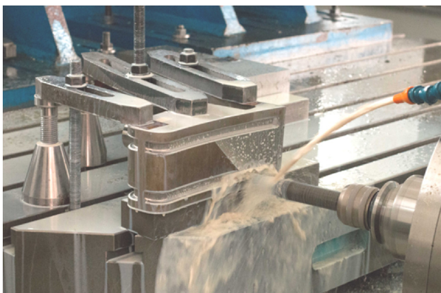
Fig. 5. Drilling of the cooling channels.
