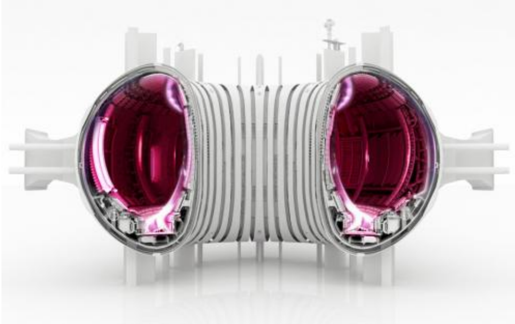
Computer-generated cutaway image of JET during a plasma experiment
