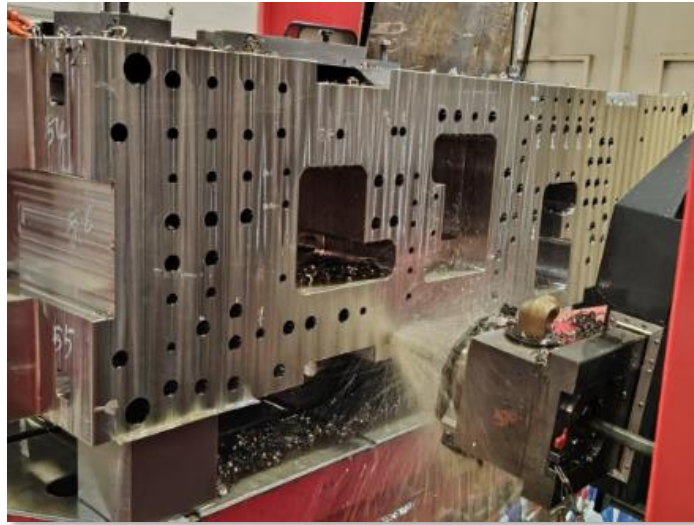
Diagnostic shield module during the gun drilling
