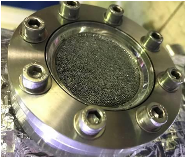
Steam exposure tests on vacuum window
