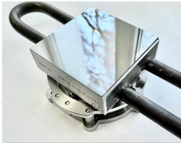
Actively cooled Molybdenum mirror
