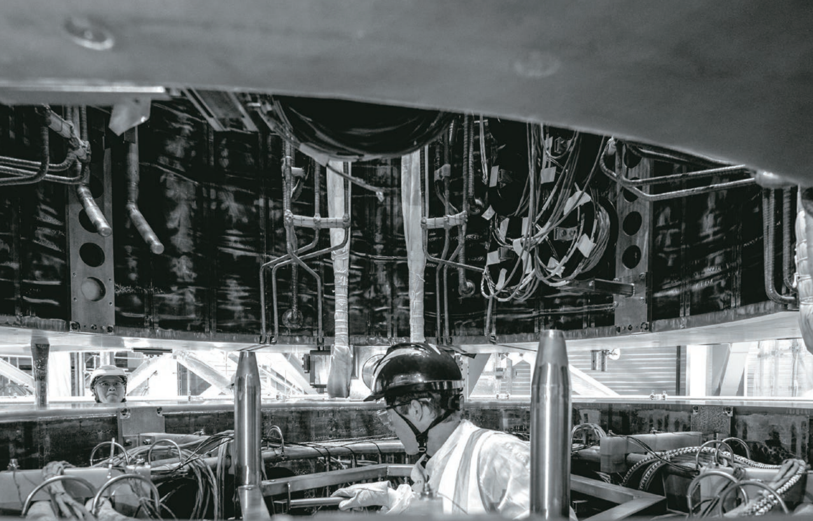
ITER personnel surveys and supervises all assembly work onsite (pictured: central solenoid assembly).
