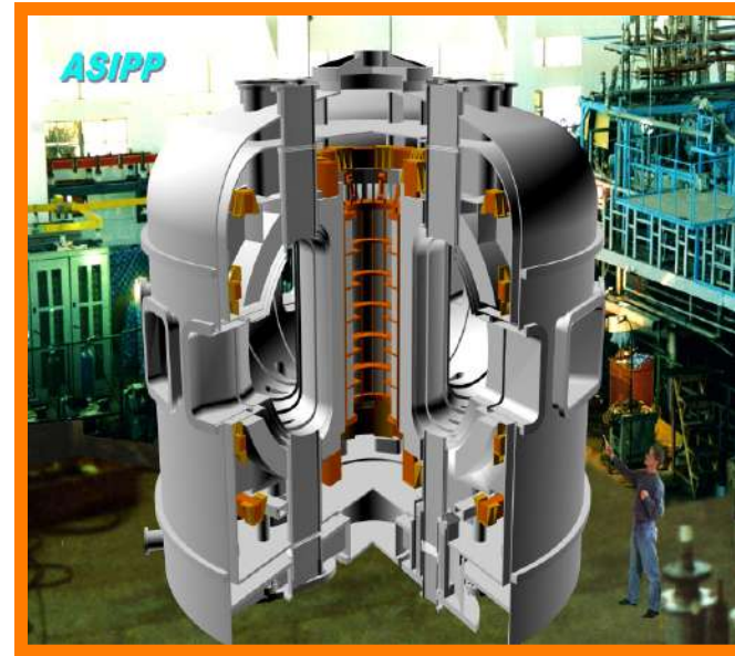
EAST China (1000 s) ( R=1.95 m, 1-1.5 MA, 4 MW, 4.6 GHz LHCD)
