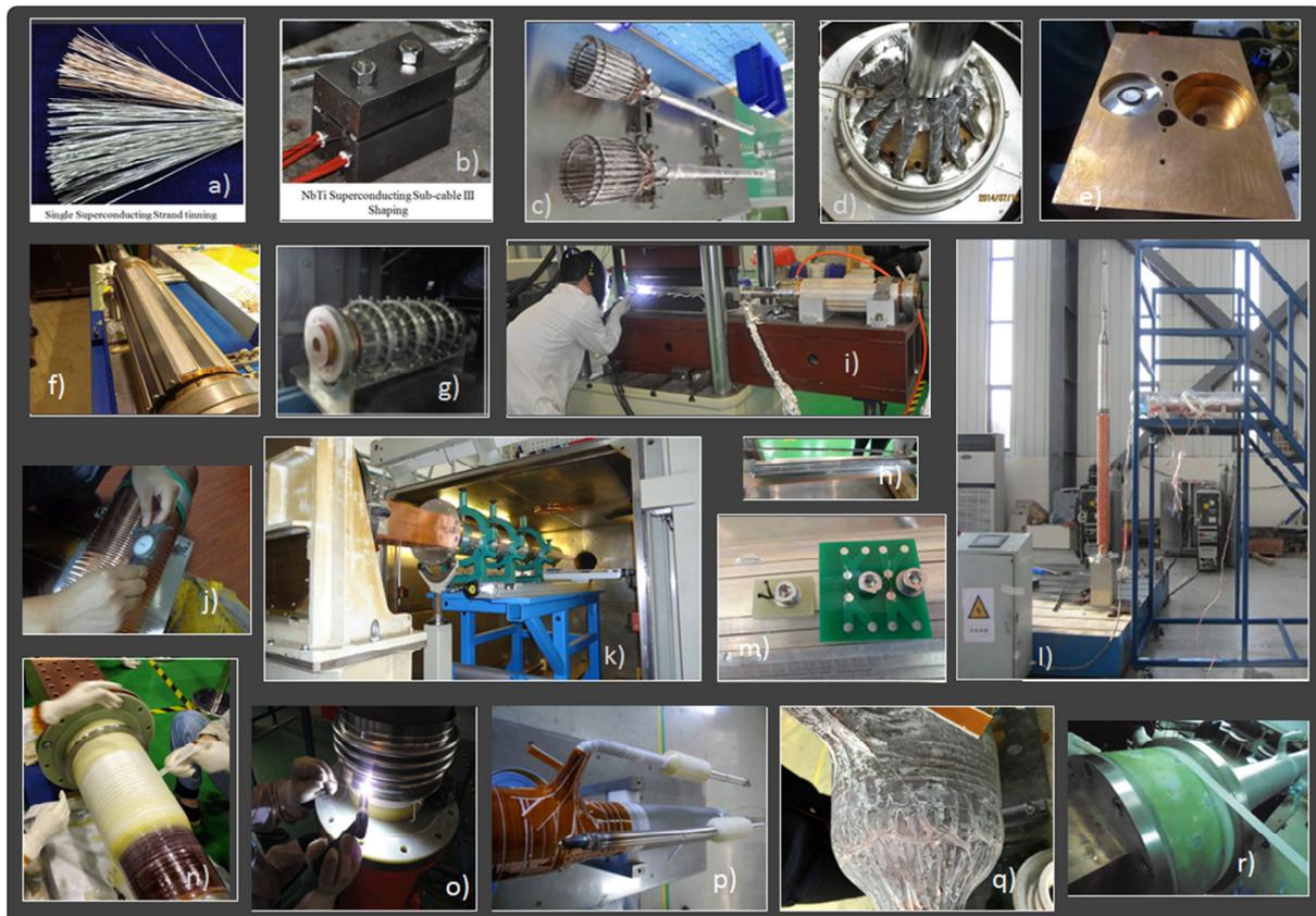
Figure 27: Prototype manufacturing. a-b): sub-cable preparation and soldering, c): LTS linker completed, d) soldering LTS linker into shunt, e) terminal brazing preparation, f) stack on shunt assembly, g) stack to shunt soldering, h) TB joint assembly i) TB joint pressure welding, j) HX geometrical testing, k) electron beam welding, l) honed tube assembly, m) mounting of temperature sensors, n) embedded ring glass wrap, o) bellows welding, p-q) main insulation, r) flange cylinder glass overwrap.
