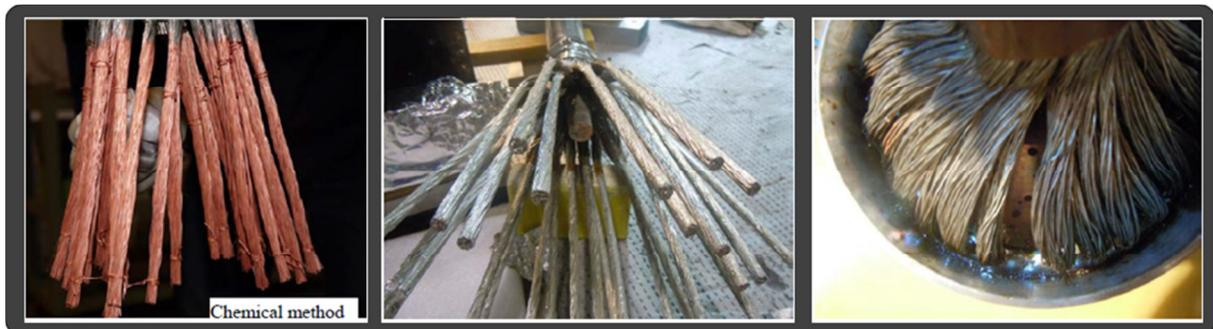
Figure 20: Preparing the sub-cables (TF-type): Left: chemical Ni removal, Middle: pre-tinning, Right: soldering into the shunt blind holes.
