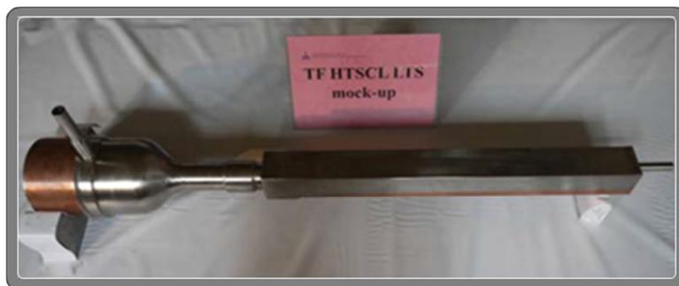
Figure 19: TF-type LTS linker mock-up (before destructive testing).
