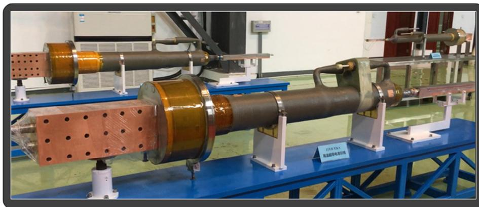
Figure 28: PF prototype lead, Background: TF prototype lead (left), CC prototype lead (right).
