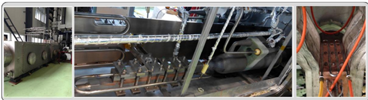
Figure 31: PF HTS-CL prototypes inserted into the test cryostat.
