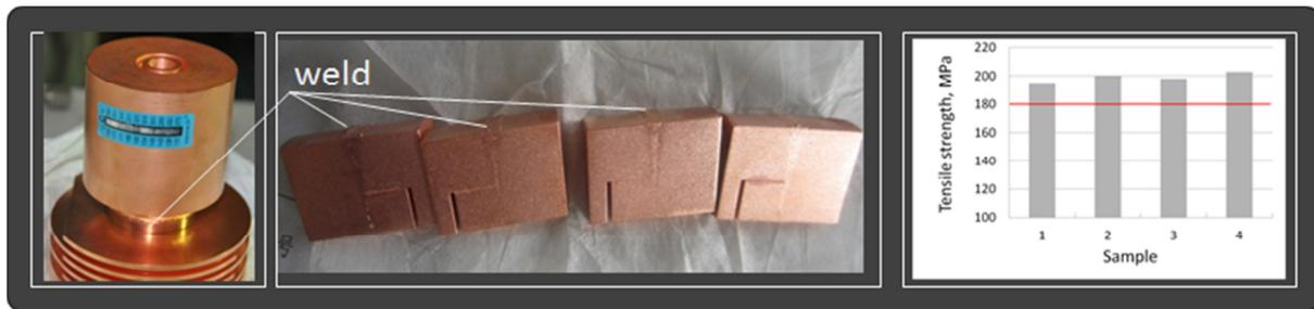
Figure 25: EBW mock-up results. Left: TF-type ebw mock-up, Middle: samples for micrographic examination of weld, Right: tensile strength measurements of weld samples.
