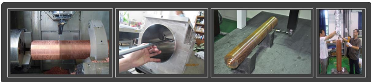
Figure 23: HX mock-up manufacturing: From left to right: HX core machining in a CNC, honed tube dimensional check with a feeler gauge, HX core dimensional check in the CMM, HX Assembly.
