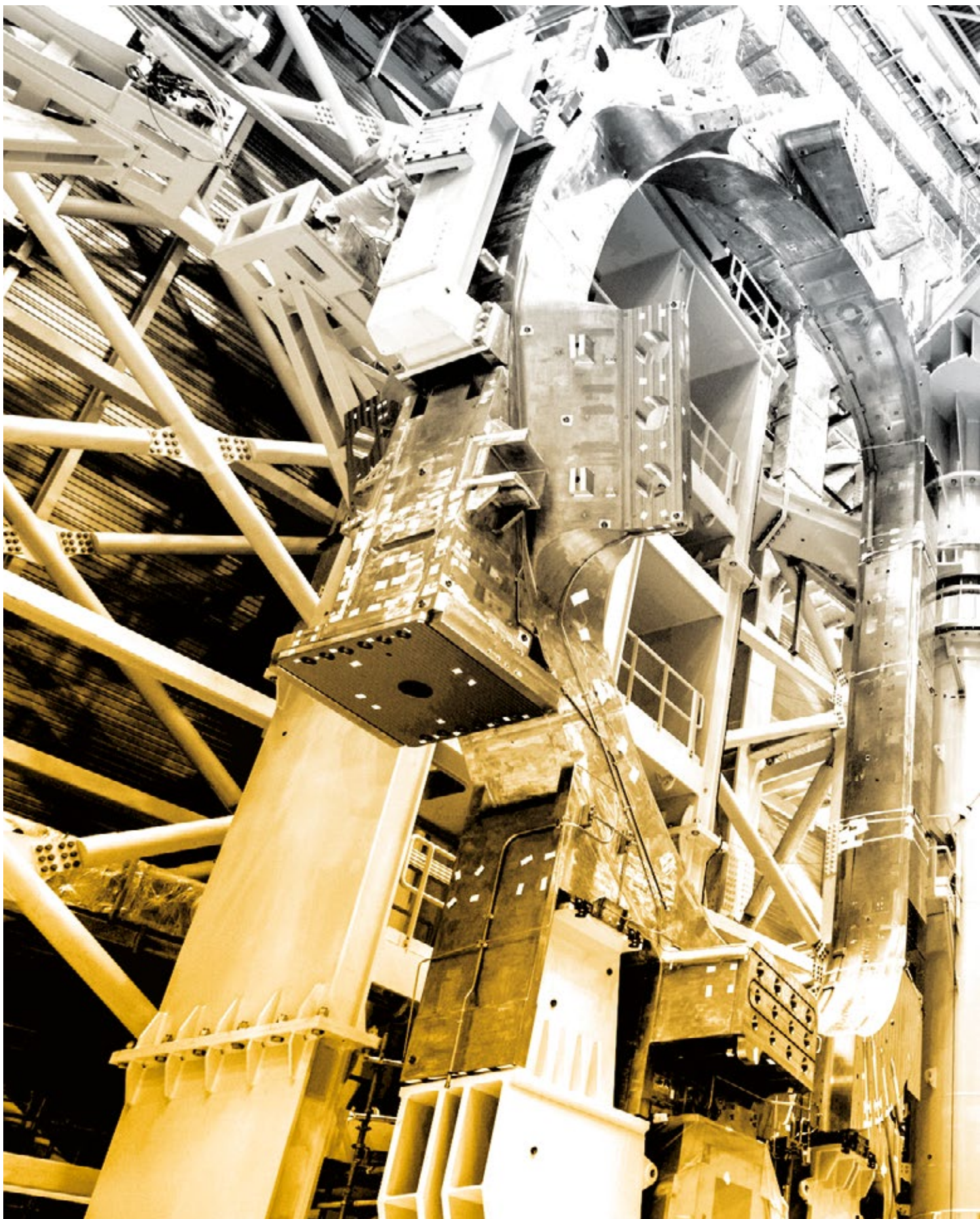
The first vacuum vessel module in construction. A module is formed from one vacuum vessel sector (440 tonnes), two D-shaped toroidal field coils (330 tonnes each), and thermal shield panels (50 tonnes).
