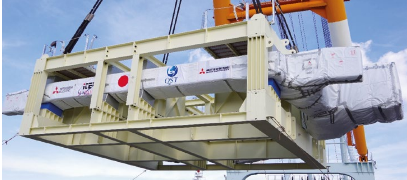
A 330-tonne, D-shaped coil travels from Japan. Eleven of the 19 toroidal field coils expected are now on site.
