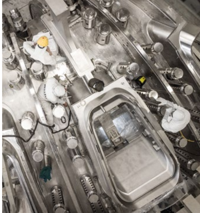
Europe is responsible for delivering five vacuum vessel sectors. Work is well advanced.
