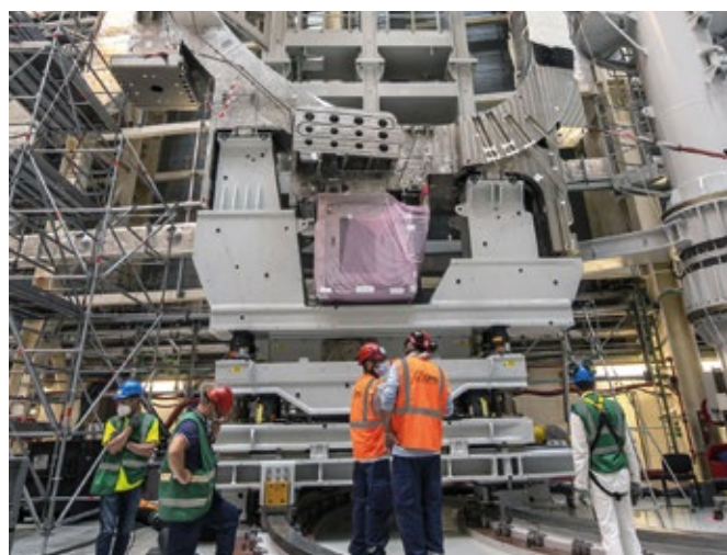
On an open wing of this sector sub-assembly tool (SSAT2), a toroidal field coil has been positioned.
