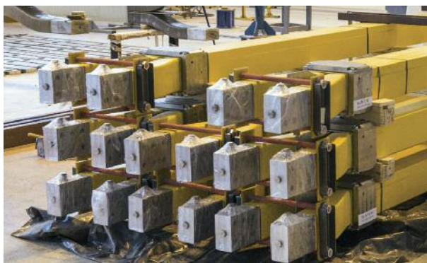
DC aluminium busbars manufactured in Russia are prepared for shipment. Over 5 km of busbars will be needed to connect ITER's superconducting magnets to their power supplies.
