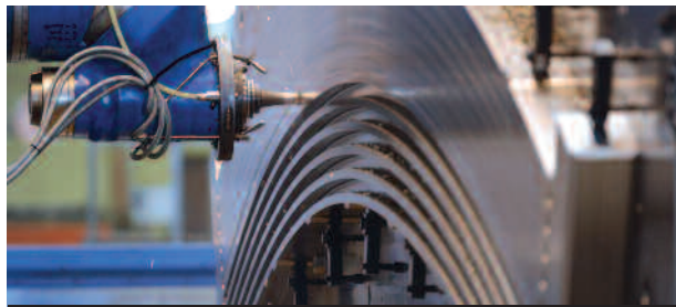
High-precision manufacturing is carried out on a "rough" stainless steel radial plate for the toroidal field coils. When assembled, the grooves will house jacketed superconducting cable. Photo: F4E
