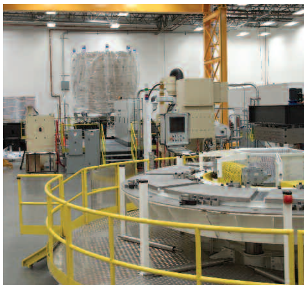
In the US, winding begins on the central solenoid mockup module that will serve to commission the production line. Photo: US ITER
