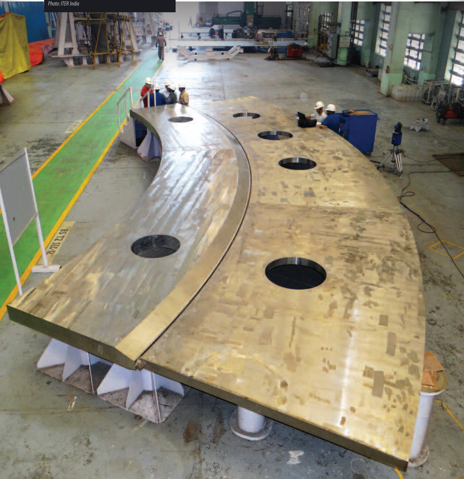
Manufacturing activities progress on the ITER cryostat in India. (Pictured: one of the six 60° segments of the cryostat base, tier 2.) Photo: ITER India
