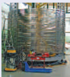
Russian-produced poloidal field cable is jacketed and compacted in Italy before being spooled to await testing and a return to Russia.
