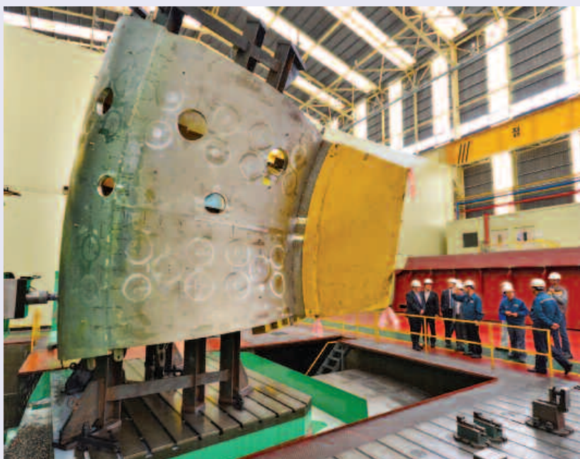
Industrial activities are progressing on two vacuum vessel sectors in Korea. Pictured: the upper segment of sector #6.
