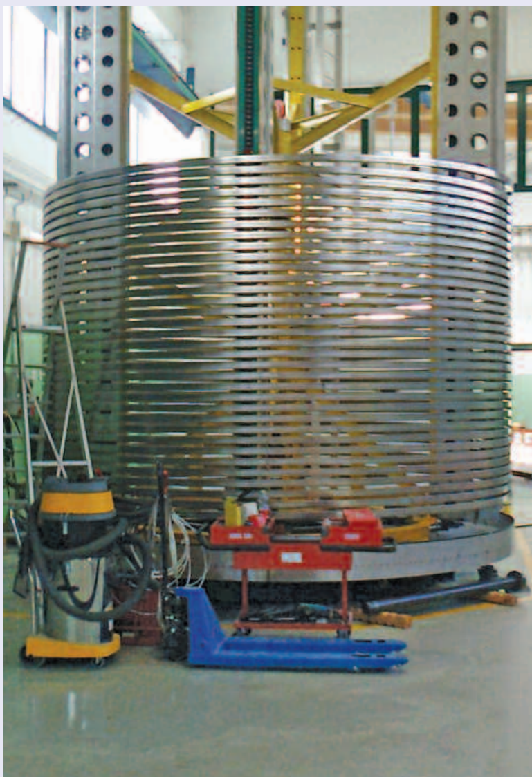
Russian-produced poloidal field cable is jacketed and compacted at Criotec (Italy) before being spooled to await testing and a return to Russia for the next stage of poloidal field coil fabrication.
