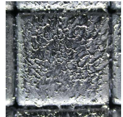
W after tests simulating 5 'Large ELMs.' Klimov PSI 2008
