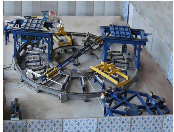
PF1 winding equipment in place in the Efremov Institute.
