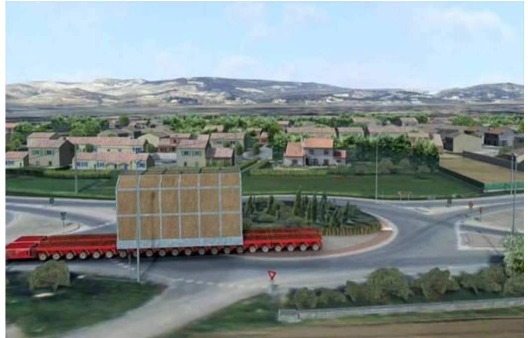
Heavy Component on Road (TF Coils, VV Sectors, and PF1 Coil)
