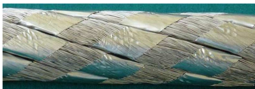
Fig. 4. Appearance of a cable after compaction.
