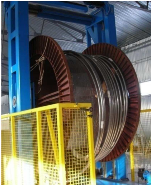
Fig. 9. Dummy conductor, 100 m, wound on the drum.
