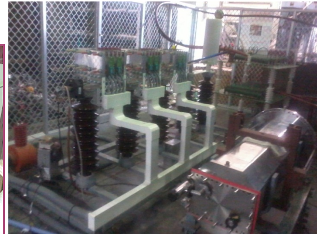
Solid state based crow bar system (Thyristor based)
