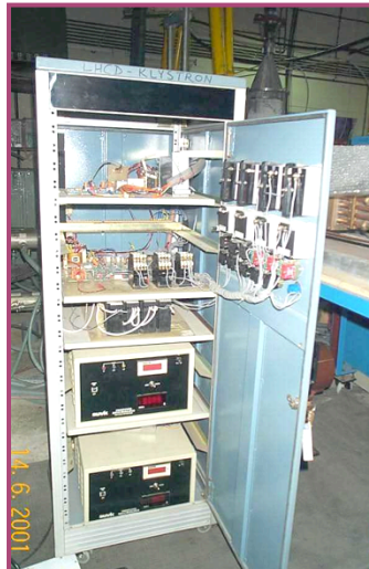
AMPS Control Panel: For synchronization if necessary and controls Tetrode, operating in its linear range.
