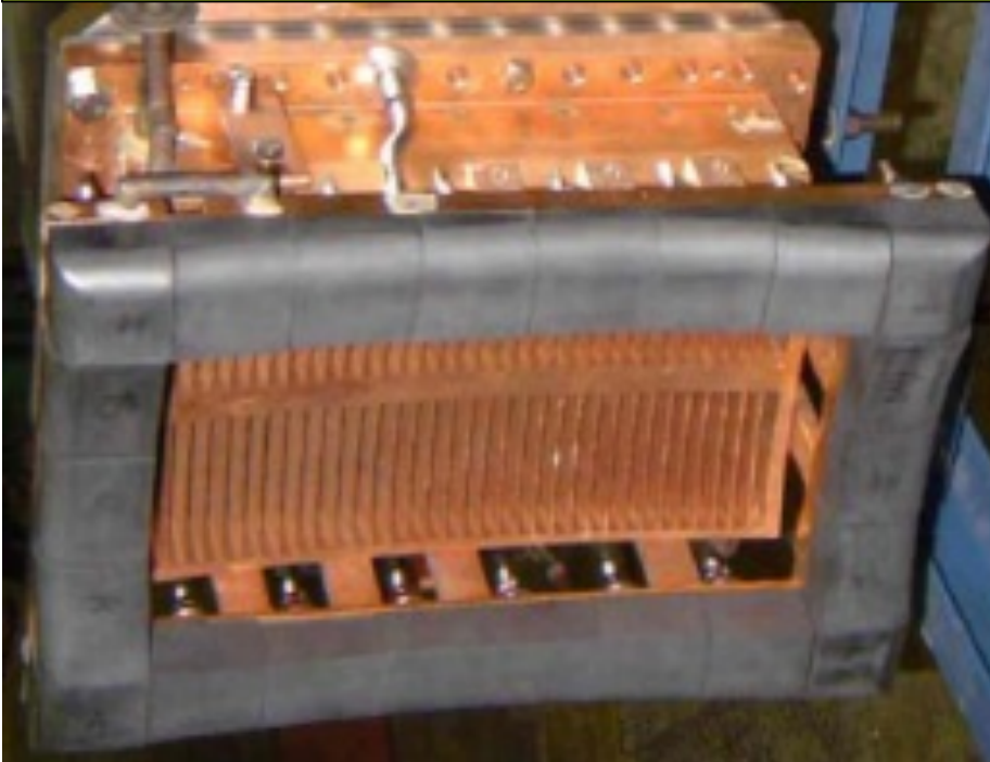
2 × 32 grill antenna for SST1 machine
