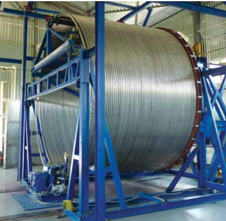
The Russian Scientific Research and Development Cable Institute JSC VNIKP completes 760 metres of copper dummy conductor as part of the qualification process for the manufacture of ITER's toroidal field conductors. Photo: RF-DA
