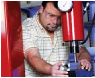
Conduit punching trials are conducted for helium penetrations on the central solenoid coils. Photo: US ITER/ORNL
