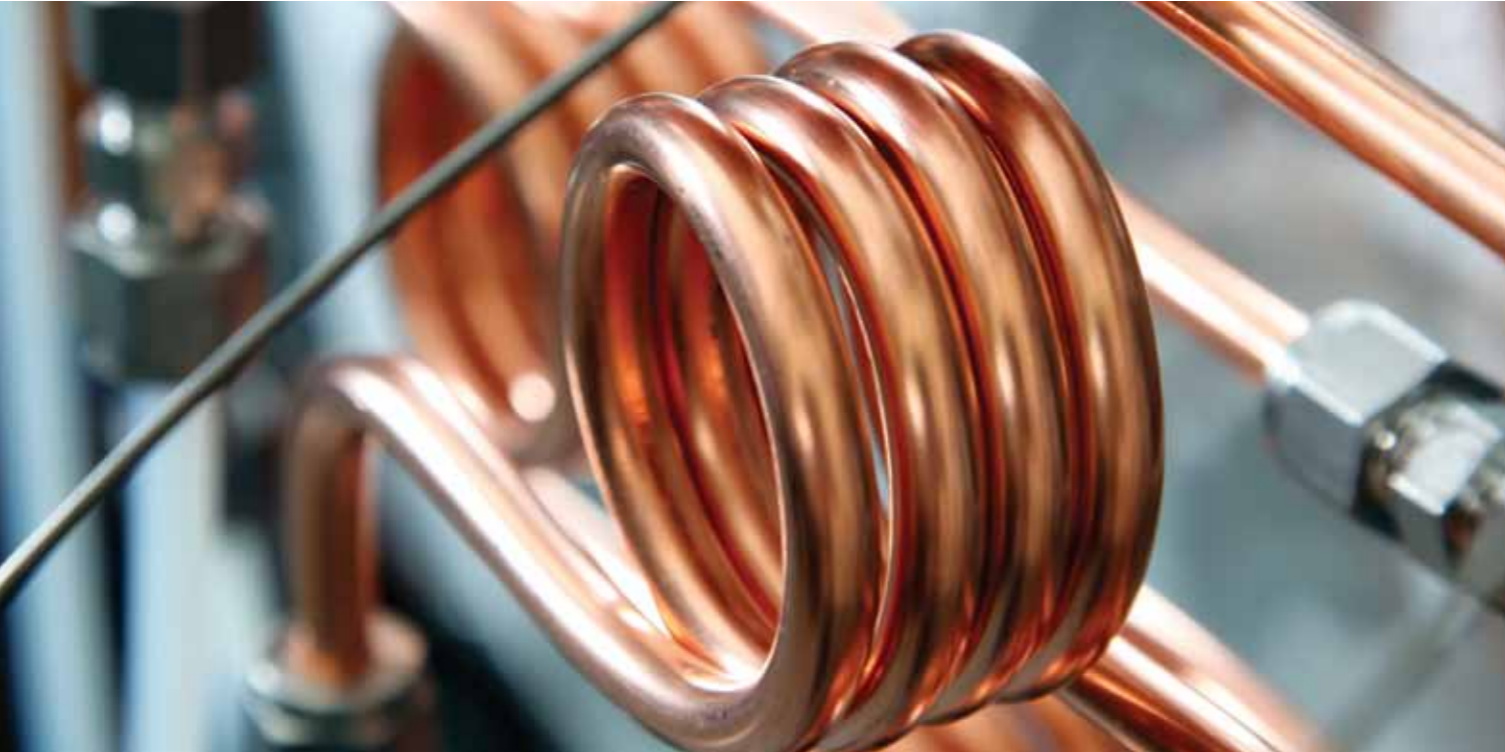
These copper cooling coils are part of a heat treatment furnace and gas management system used by US ITER to prepare samples of critical superconducting components for ITER magnets. Photo: US ITER/ORNL
