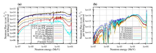
**Figure 3.** Comparison of the neutron-energy spectra in DEMO; (a) as a function of depth into the vessel from the plasma-facing wall at the equatorial position A in figure 2; and (b) in the first two layers of the divertor as a function of position (E–G in figure 2).
