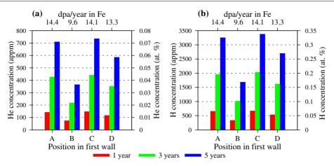
**Figure 5.** Variation in the (a) He, and (b) H, concentrations in pure Fe as a function of time for the spectra at different FW armour positions in DEMO—see figure 2. The equivalent dpa/year in pure Fe at each position are also given.
