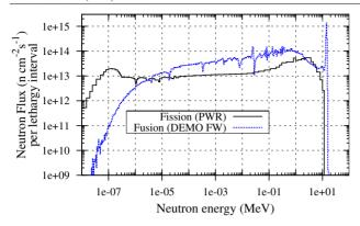
**Figure 1.** Comparison of the neutron-energy spectra in fission and fusion reactors. For fission the average neutron spectrum in the fuel assembly of a PWR reactor is shown, while the equatorial FW armour spectrum for the DEMO model in figure 2 is representative of fusion.
