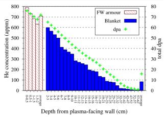
**Figure 7.** Variation in He concentration in pure Fe after a five-year irradiation as a function of depth (from the plasma) into the FW armour and blanket of DEMO at A in figure 2. The total dpa in pure Fe at each depth after five years is also shown (pluses).
