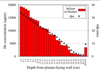
**Figure 9.** Variation in He concentration in pure Be after a five-year irradiation as a function of depth into the DEMO blanket at (A) in figure 2. The equivalent dpa in pure Be after five years is also given at each depth.
