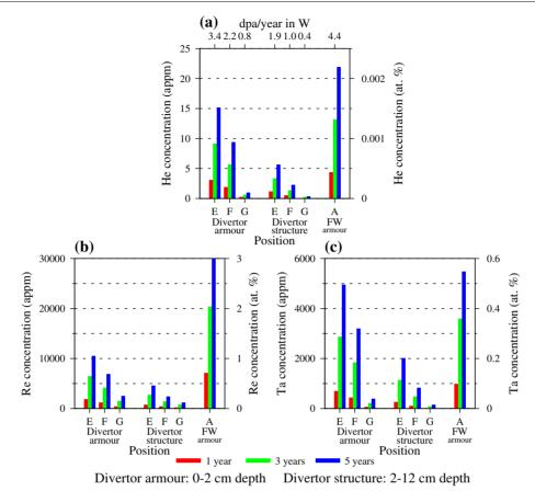
**Figure 8.** Variation in concentrations of (a) He, (b) Re and (c) Ta, produced in pure W under neutron irradiation as a function of position (and depth) in the divertor region of the DEMO design (figure 2). In (a) the equivalent dpa year $^{-1}$  in pure W are also given for each position.
