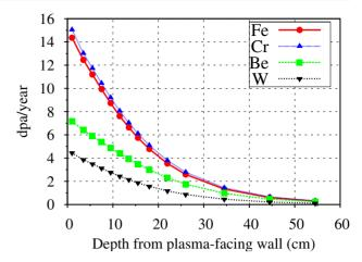
**Figure 4.** Defect production rates, expressed in dpa per year units for different elements shown as a function of depth into the FW armour and blanket at A in figure 2.
