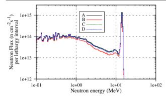
**Figure 6.** The high-energy part of the neutron spectra for the 2 cm FW armour layer at four different positions within the DEMO model (figure 2). The slight drop in the flux at B shown here leads to the  $\sim$ 50% drop in gas production in figure 5.
